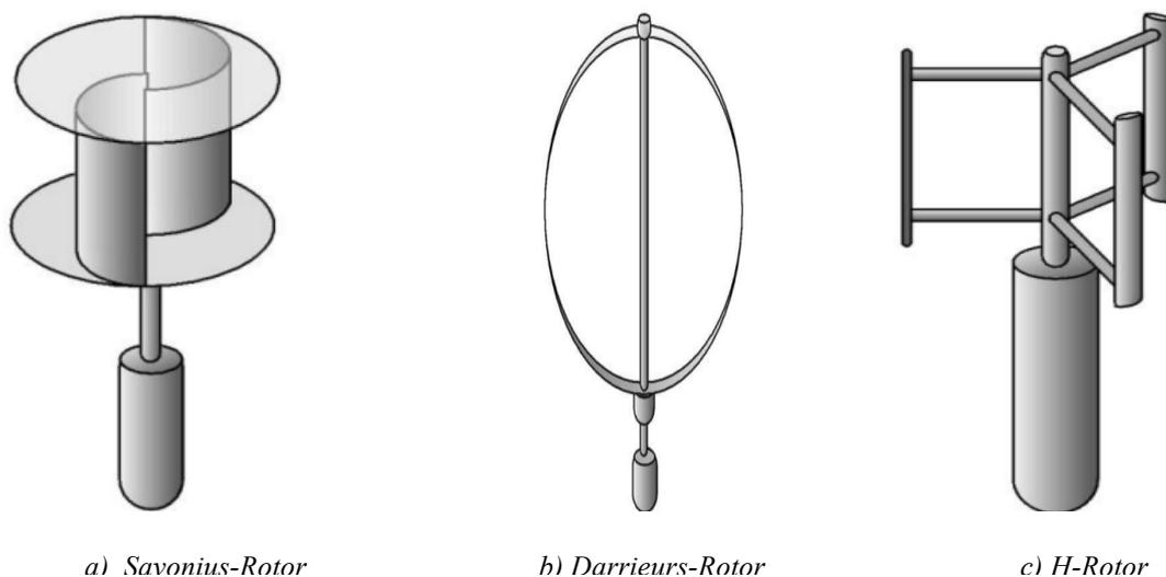
**Figure 5:** Three different types of vertical axis turbines[65].
