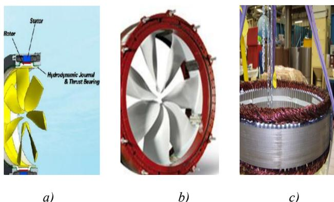
**Figure 9:** a) Arrangement of the electrical machine on the periphery of the propeller of a propellant Bow,
