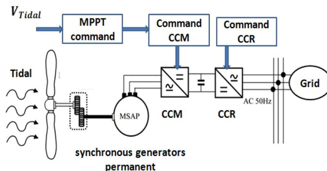
Figure 7: The connection of a tidal turbine system to the power via PMSG.
