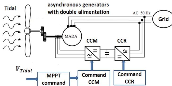
Figure 6: The connection of a tidal turbine system to the power grid via a DFIG.
