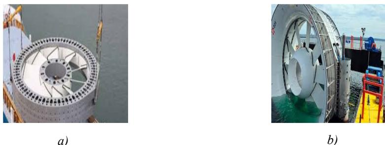
**Fig. 10:** a) View of the OpenHydro hydro-turbine rotor (500kW),
