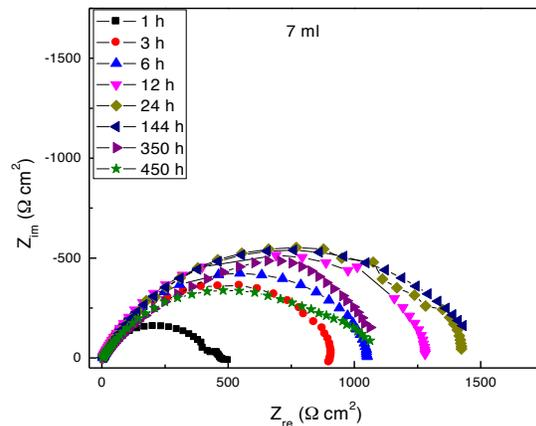
**Figure 5:** Nyquist diagrams at different exposure times for 1018 carbon steel in 0.5 M H<sub>2</sub>SO<sub>4</sub> solution containing 7 ml of *L. edodes*.
