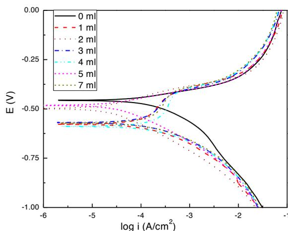
**Figure 2:** Effect of the polarization curves for 1018 carbon steel in 0.5 M H<sub>2</sub>SO<sub>4</sub>.
