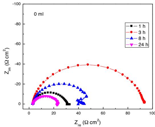
**Figure 4:** Nyquist diagrams at different exposure times for 1018 carbon steel in uninhibited 0.5 M H<sub>2</sub>SO<sub>4</sub> solution.
