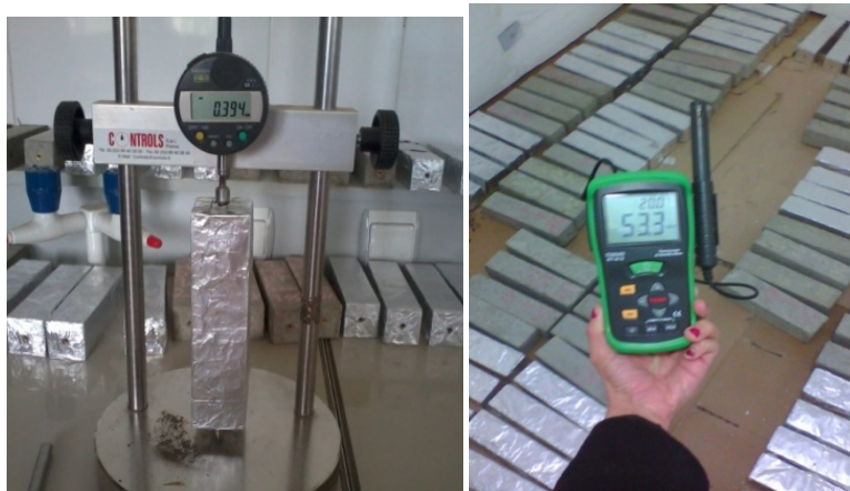
Figure 17: Device for measuring endogenous shrinkage formations
