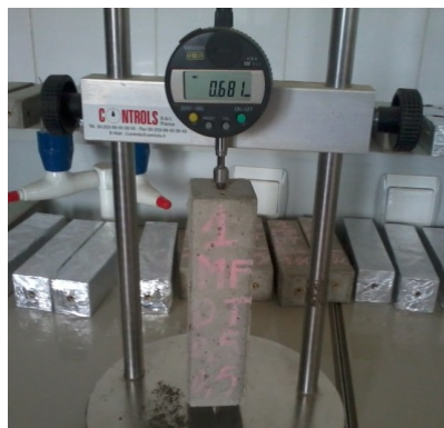
Fig. 13: Device for measuring the shrinkage formations in desiccation mode
