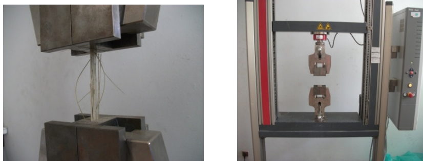
Figure 9: Mounting used for direct fiber pull test
