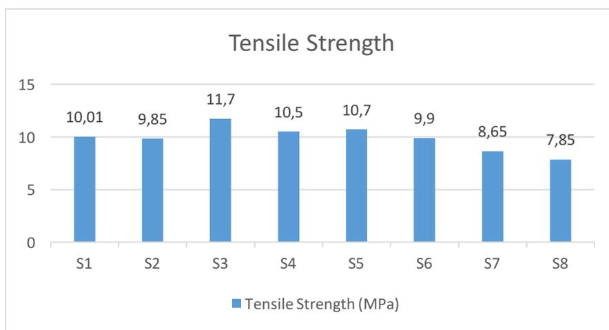
**Figure 1:** Variation of Tensile Strength of Samples
