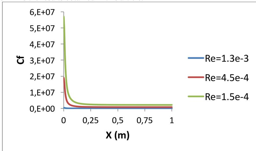
**Figure 4:** Surface Friction Coefficient profile along the vertical wall for the volume fraction of 7% of nanoparticles (Nanofluids  $Al_2O_3$ /Propellant Dough(35/45)) – the fluid temperature of 20°C and temperature difference of fluid and wall 24°C and  $n=0.440$
