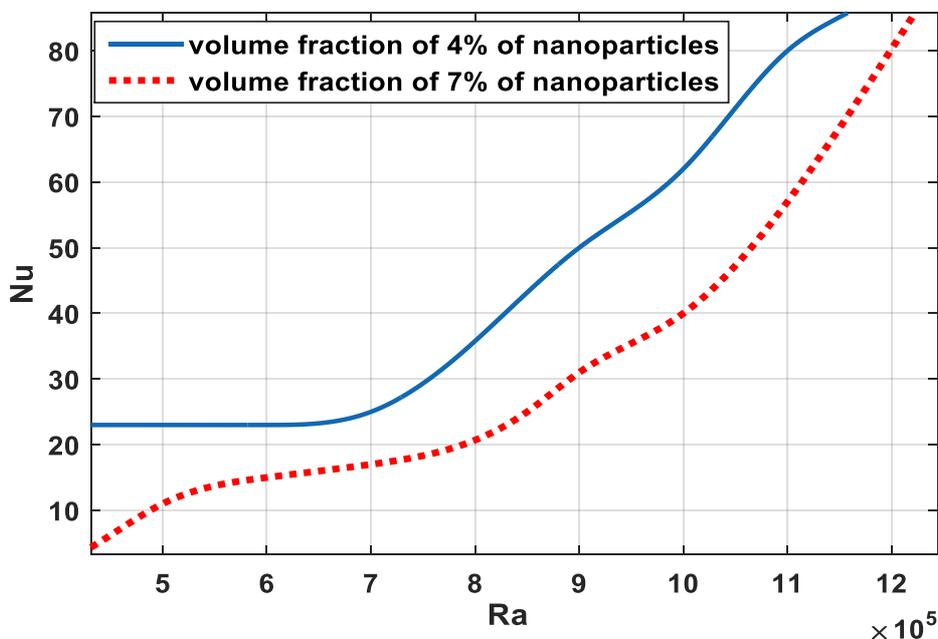
**Figure 6:** Nusselt number profile along the vertical wall according to Rayleigh number for the volume fraction of 4% and 7% of nanoparticles (Nanofluids  $\text{Al}_2\text{O}_3/\text{Propellant Dough}(35/45)$ ) –  $n=0.440$
