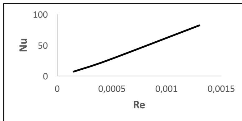
**Figure 2:** The Average Nusselt Number Profile in the length of the vertical wall according to Reynolds number for the volume fraction of 7% of nanoparticles (Nanofluids  $Al_2O_3/Propellant\ Dough(35/45)$ ) – the fluid temperature of  $20^\circ C$  and temperature difference of fluid and wall  $24^\circ C$  and  $n=0.440$
