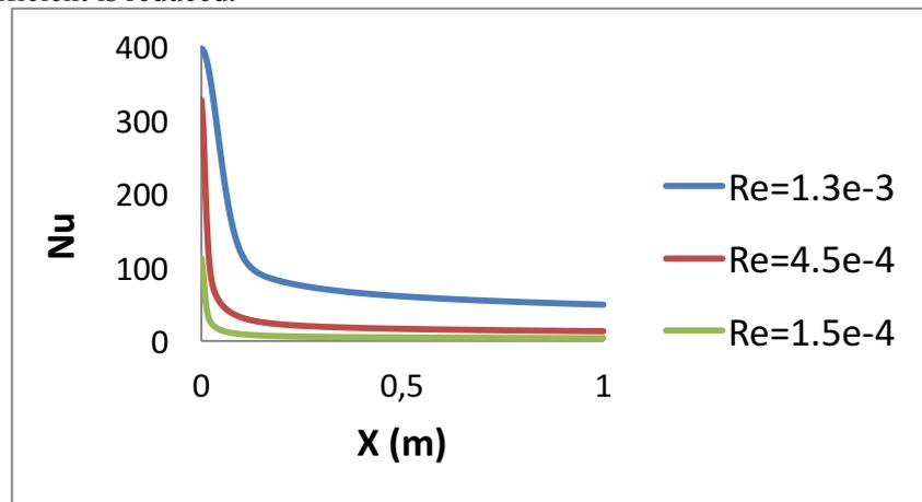
**Figure 1:** Nusselt number profile along the vertical wall for the volume fraction of 7% of nanoparticles (Nanofluids  $Al_2O_3/Propellant\ Dough(35/45)$ ) – the fluid temperature of  $20^\circ C$  and temperature difference of fluid and wall  $24^\circ C$  and  $n=0.440$
