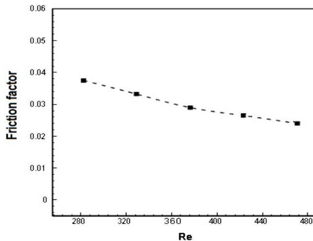
**Figure 5:** Surface Friction Coefficient Profile according to Reynolds numbers for a nanofluid [10]
