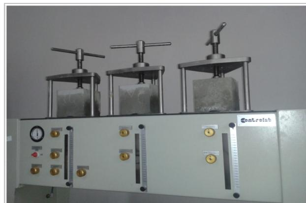
**Figure 3:** Water penetration test setup
