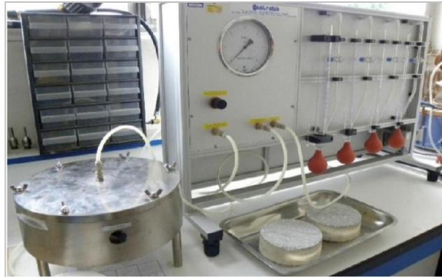
**Figure 2:** General view of CEMBUREAU gas permeameter
