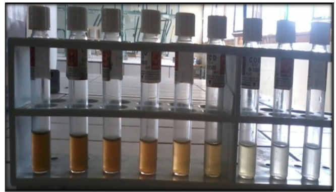
Figure 4: Discoloration of OMW during electrolysis at 100mA/cm 2
