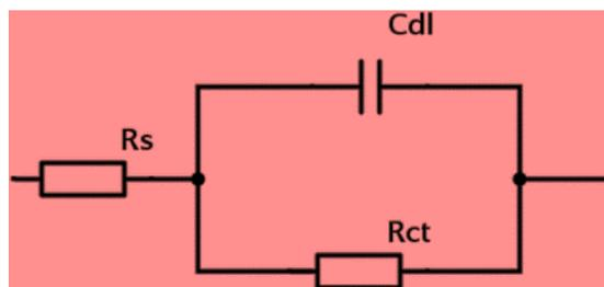
Fig.i Randle's equivalent circuit
