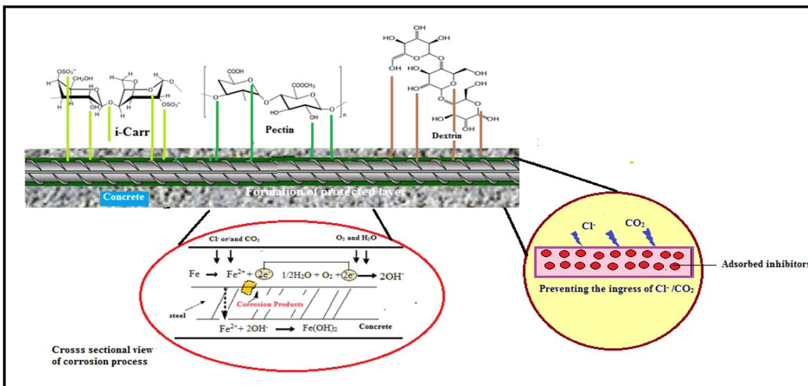
Fig.10 Pictorial representation of mechanism of rebar corrosion
