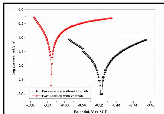
**Fig. 5** Polarization plots of pore solution with and without chlorine
