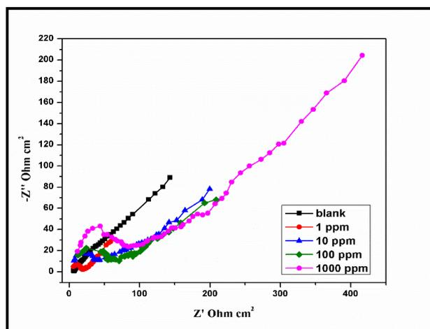
**Fig. 4** Nyquist plot of Dex for corrosion of rebar
