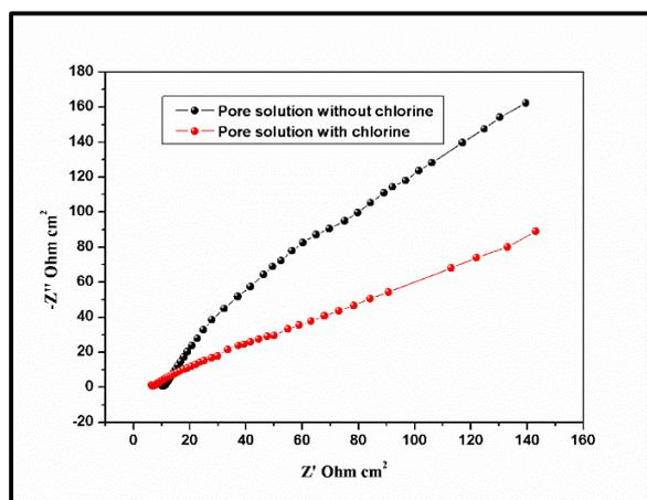
**Fig. 1:** Nyquist plots of pore solution with and without chlorine
