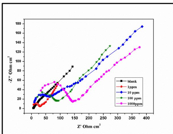
**Fig. 2** Nyquist plot of i-Carr for corrosion of rebar
