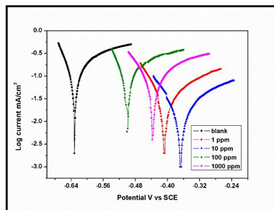
Fig. 6 Polarization plots of  $i_{\text{Corr}}$  for corrosion of rebar Fig. 7. Polarization plots of  $P_{\text{ec}}$  for corrosion of rebar
