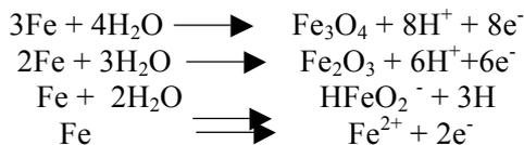
The cathodic reactions probably depends on the accessibility of O<sub>2</sub> and pH of the pore solution adjacent to the steel surface. The most expected reactions are as follows
