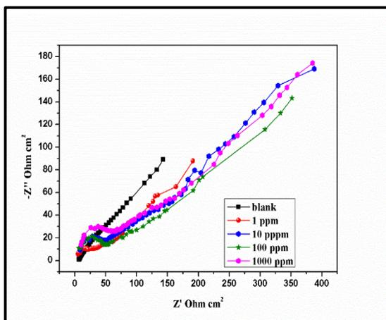
**Fig. 3** Nyquist plot of Pec for corrosion of rebar
