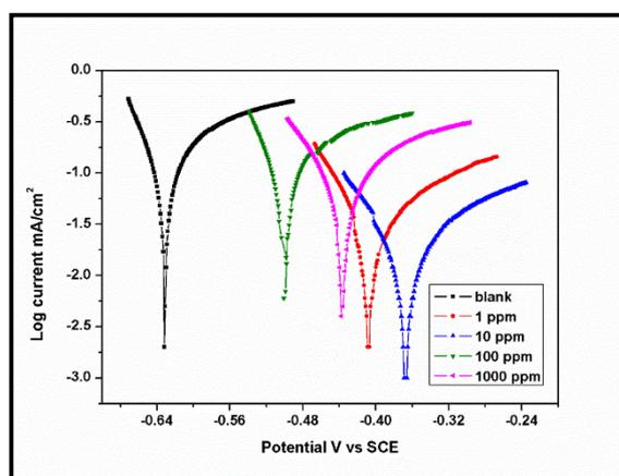
Fig. 8 Polarization plots of  $D_{\text{ex}}$  for corrosion of rebar
