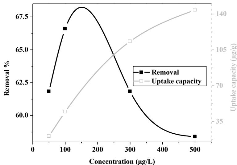
**Figure 1:** Effect of initial arsenic concentration on the biosorption of As(V) (Experimental conditions: dose = 0.15 g; contact time = 20 min; pH = 6.0; temperature = 25 °C; agitation speed = 300 rpm).
