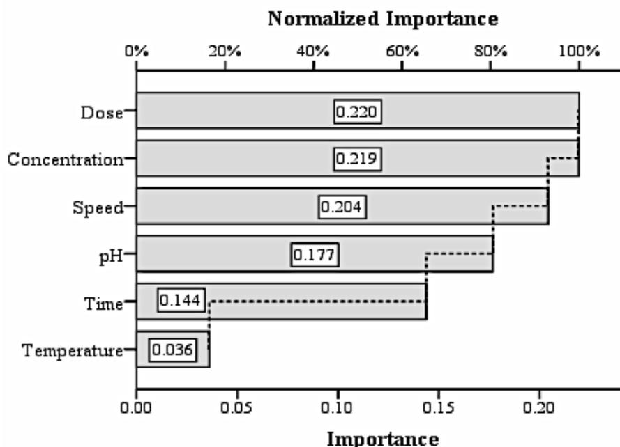
**Figure 10:** Effect of various experimental (input) parameters on biosorption efficiency.
