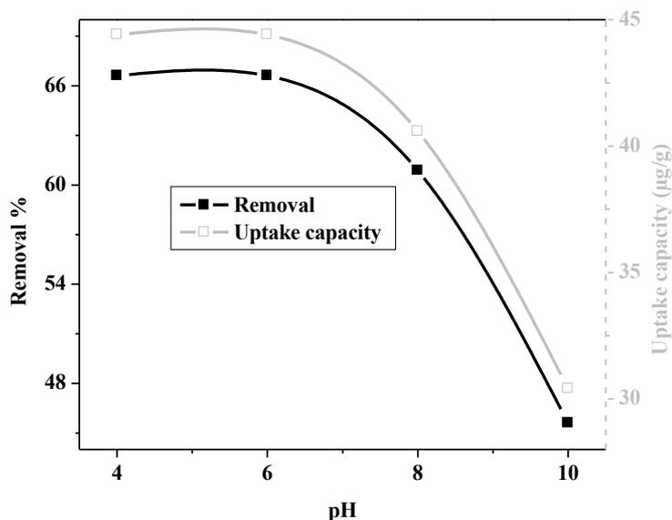
**Figure 2:** Effect of pH on the biosorption of As(V) (Experimental conditions: initial arsenic concentration = 100 μg/L; dose = 0.15 g; contact time = 20 min; temperature = 25 °C; agitation speed = 300 rpm).
