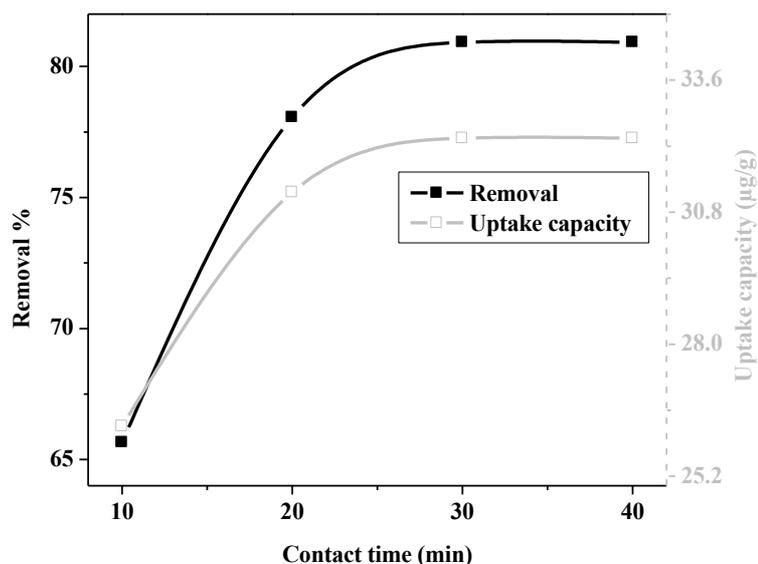
**Figure 4:** Effect of contact time on the biosorption of As(V) (Experimental conditions: initial arsenic concentration = 100  $\mu\text{g/L}$ ; dose = 0.25 g; pH = 6.0; temperature = 25  $^{\circ}\text{C}$ ; agitation speed = 300 rpm).
