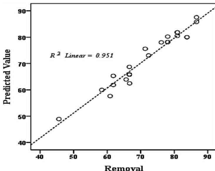
**Figure 8:** Comparison of the experimental data with those predicted by ANN model [As(V) removal].
