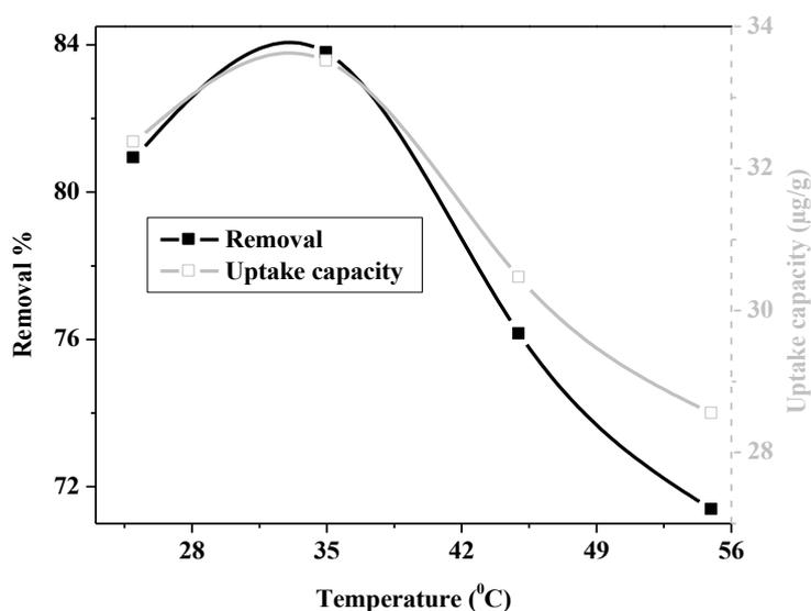
**Figure 5:** Effect of temperature on the biosorption of As(V) (Experimental conditions: initial arsenic concentration = 100 μg/L; dose = 0.25 g; contact time = 30 min; pH = 6.0; agitation speed = 300 rpm).
