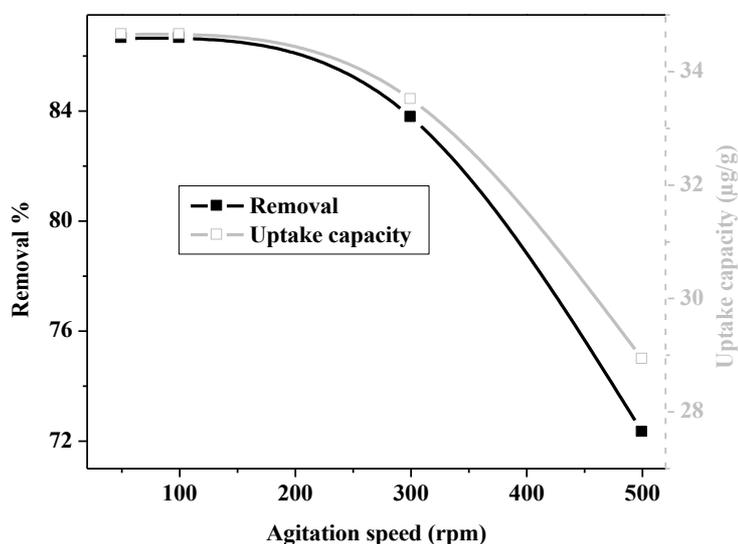
**Figure 6:** Effect of agitation speed on the biosorption of As(V) (Experimental conditions: initial arsenic concentration = 100 μg/L; dose = 0.25 g; contact time = 30 min; pH = 6.0; temperature = 35 °C).
