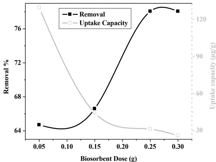
**Figure 3:** Effect of biosorbent dose on the biosorption of As(V) (Experimental conditions: initial arsenic concentration = 100  $\mu\text{g/L}$ ; contact time = 20 min; pH = 6.0; temperature = 25  $^{\circ}\text{C}$ ; agitation speed = 300 rpm).
