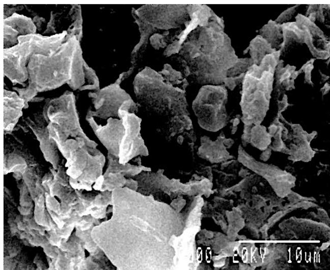
**Figure 11:** SEM micrograph of AiBP before treatment.
