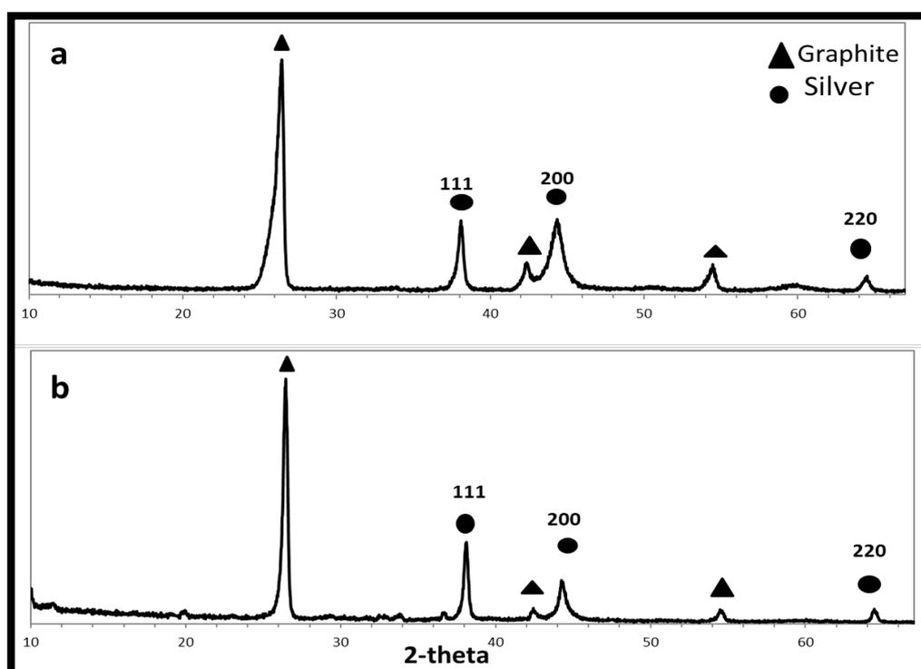
**Fig. 10 :**XRD pattern of Ag/C catalyst prepared by (a) double-pulse,(b) Pulsed current electrodeposition techniques
