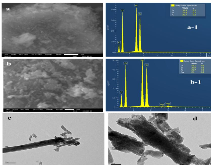
Figure 2: SEM images of (a) HNT, (b) HNT/GT/Ag-NPs and their EDS spectra of (a-1) HNT and (b-1) HNT/GT/Ag-NPs and TEM images of (c) HNT and (d) HNT/GT/Ag-NPs
