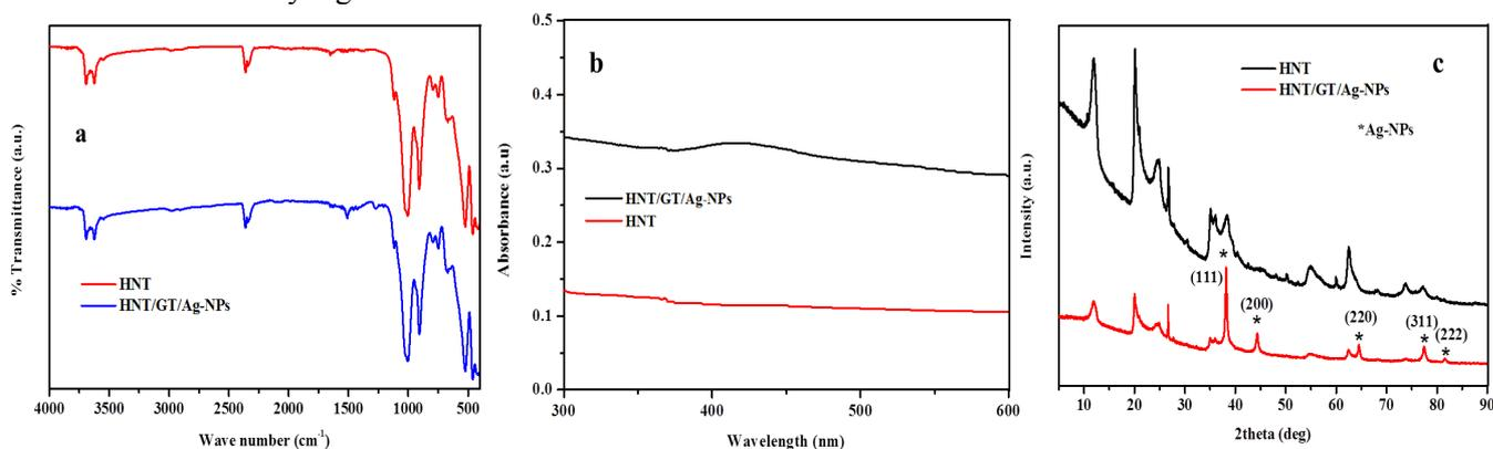
**Figure 1:** (a) FTIR, (b) UV-Visible spectra and (c) XRD patterns of HNT and HNT/GT/Ag-NPs
