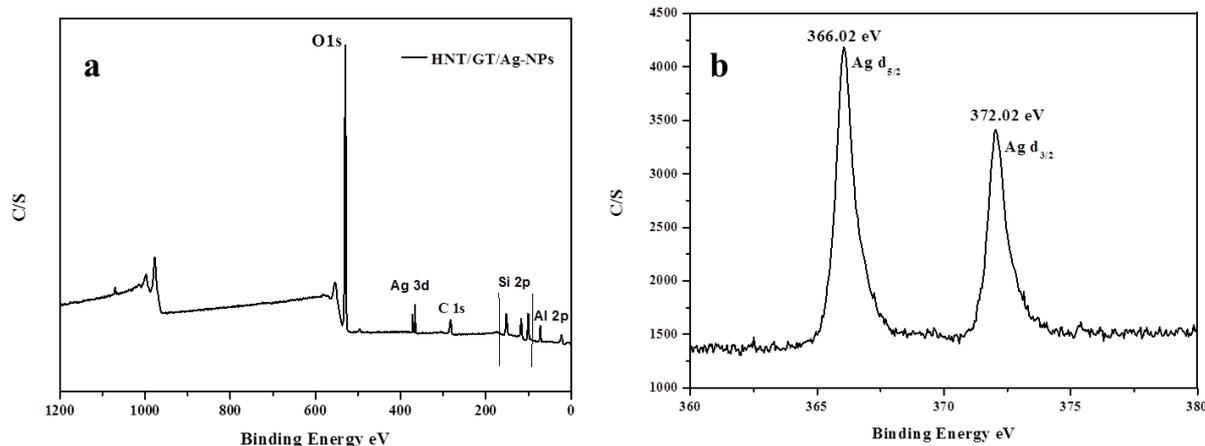
**Figure 3:** XPS spectra of (a) HNT/GT/Ag-NPs and (b) Ag 3d region
