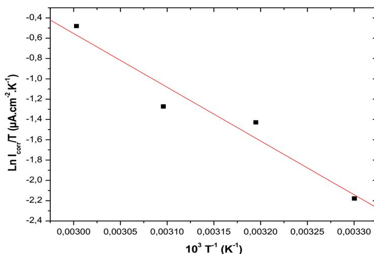
**Figure 13:** Arrhenius plots of  $\text{Ln } I_{\text{corr}}/T = f(1/T)$  for steel in 1M HCl in the absence and the presence of [Pr] extract at optimum concentration
