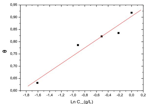
**Figure 7:** Langmuir's adsorption isotherm of [Pr] extract on the C-steel surface in HCl solution
