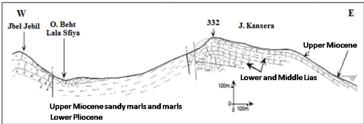
Figure 5: Geological cross-section of Jbel El Kansera [15].
