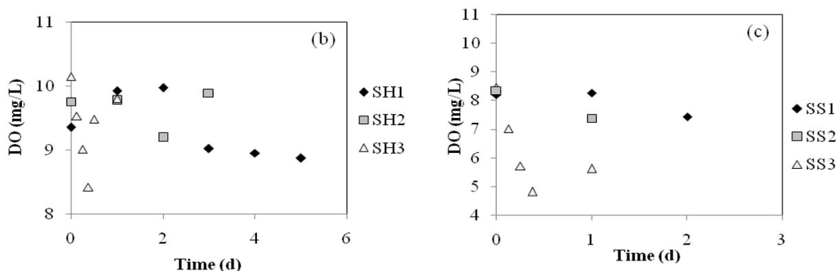
**Figure 9 :** Dissolved oxygen evolution SH and SS
