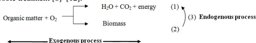
Figure 1: Removal biological process of organic matter
