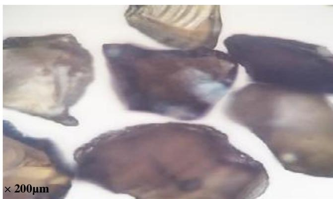
**Figure 2:** Morphology of the SiC particles using in abrasion-corrosion
