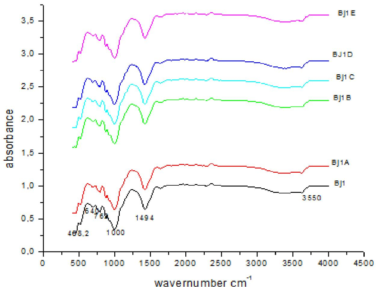
**Figure 6:** IR spectra of Bj1 and mixtures of Bj1 /cellulose / pozzolan.
