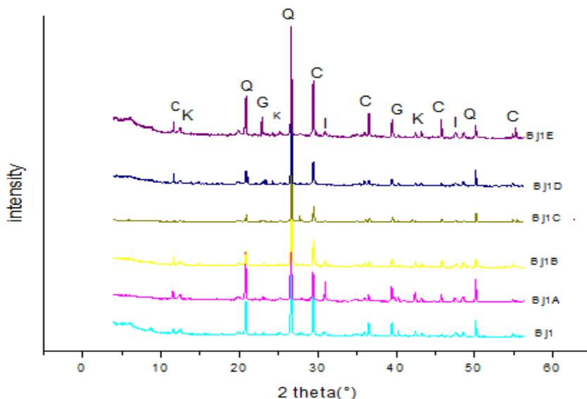
**Figure 2:** RX Diffractograms of the raw sample Bj1 and mixtures of Bj1 /cellulose / pozzolan.
