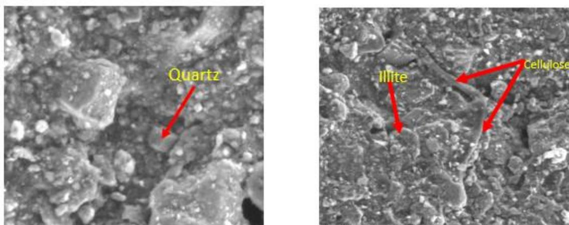
**Figure 5:** Microphotographs of a mixture of Bj1 /cellulose / pozzolan.
