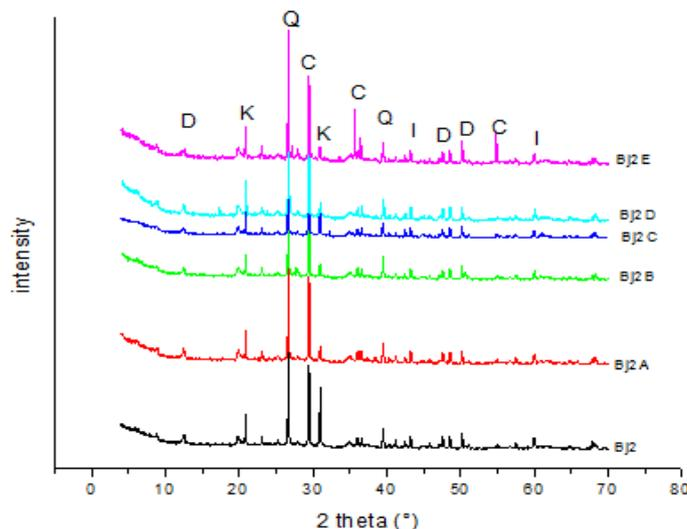
**Figure 3:** RX Diffractograms of the raw sample Bj2 and mixtures of Bj2 /cellulose / pozzolan
