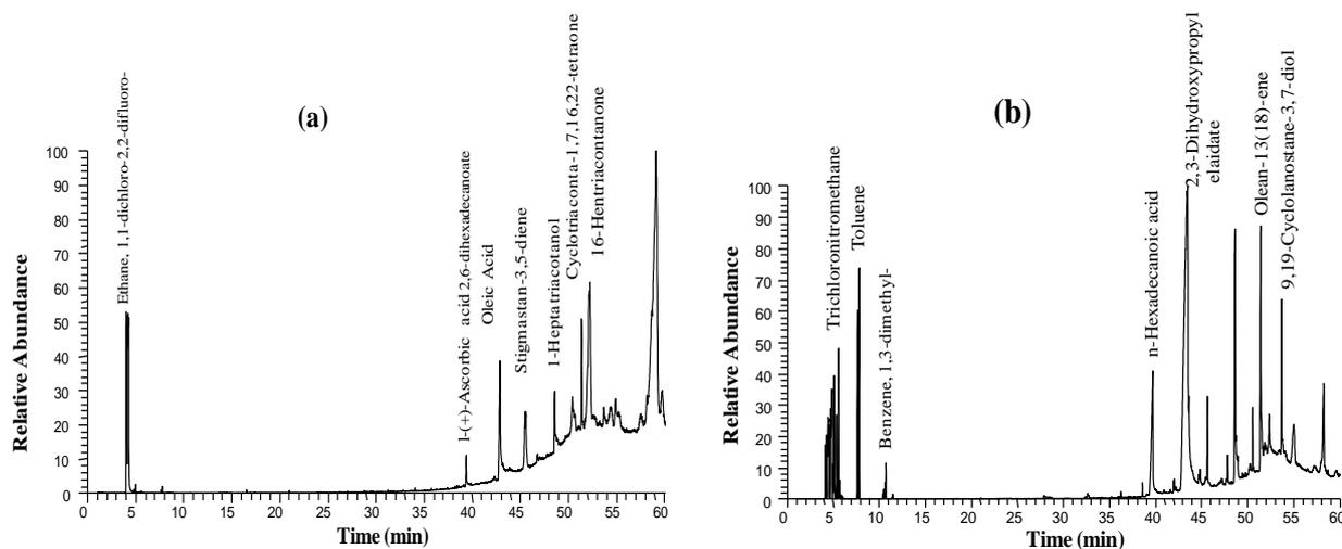
**Figure 2:** Main organic components of the Mediouna landfill leachate detected by GC-MS chemical extraction with (a) dichloromethane and (b) hexane
