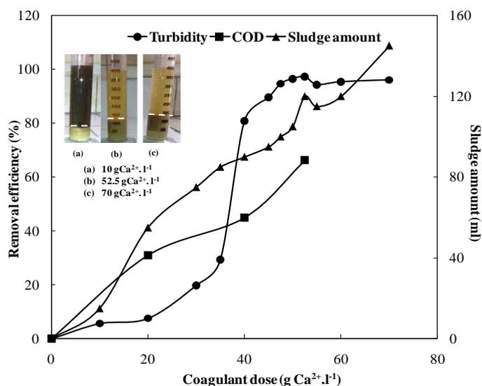
**Figure 3:** Effect of lime dosages on removal efficiency in terms of turbidity, COD and sludge amount.
