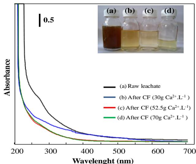
**Figure 4:** Colour variation and UV-vis absorbance spectra of the landfill leachate before and after the coagulation-flocculation-sedimentation treatment by the lime coagulant
