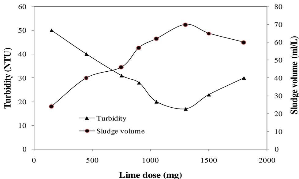
**Figure 1c:** Evolution of turbidity and sludge volume depending on the dose of  $\text{Ca}(\text{OH})_2$
