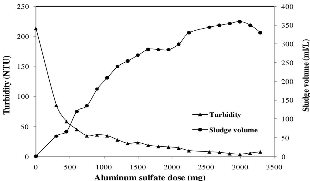
Figure 1a: Evolution of turbidity and sludge volume depending on the dose of  $\text{Al}_2(\text{SO}_4)_3$
