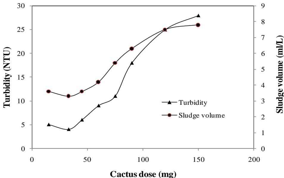
**Figure 1d:** Evolution of turbidity and sludge volume depending on the dose of Cactus
