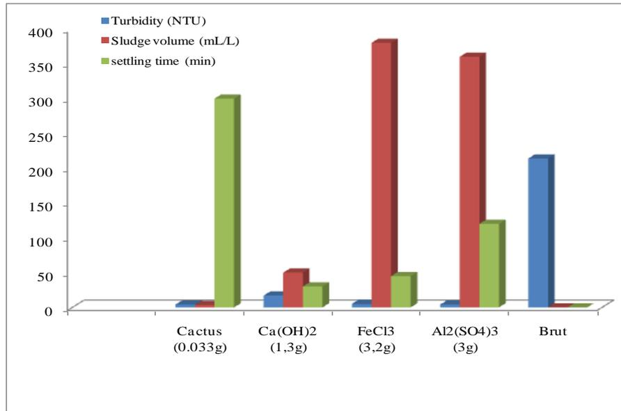
**Figure 2:** Evolution of the turbidity, the volume of sludge and the settling time according to the type of coagulants
