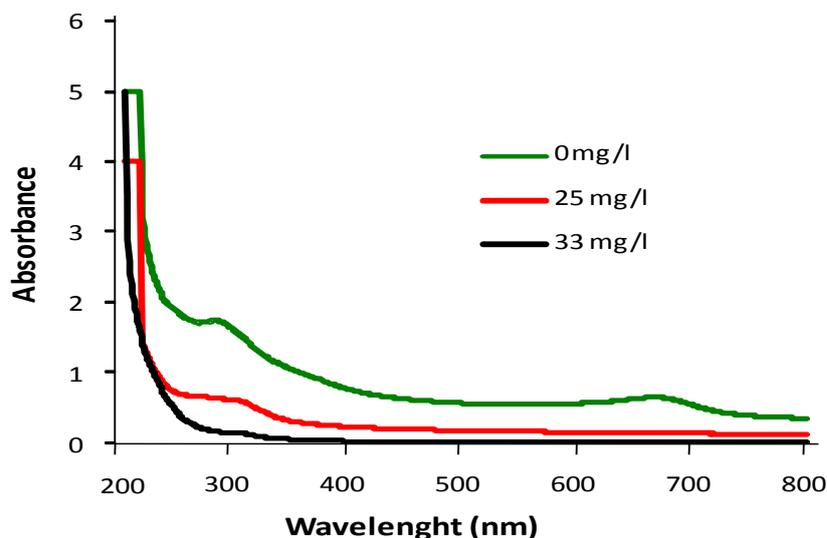
**Figure 3:** UV-vis absorbance spectra of the raw effluent and treated with cactus
