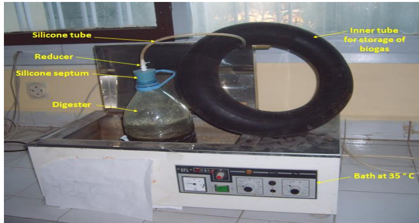
Figure 1: Experimental device for monitoring the methane fermentation of these two organic wastes
