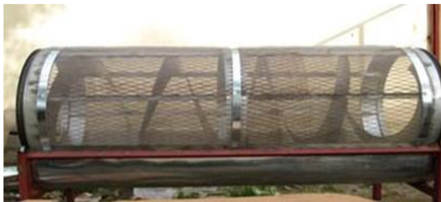
Figure 2: cylindrical composter for maturation of methacomposts
