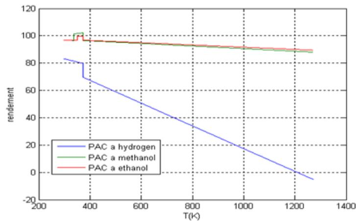
**Figure 9 :** Influence of temperature on the reversible yield of FC (P = 1atm Pure Oxygen)
