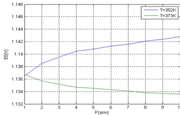
**Figure 2 :** The pressure effect on EMF of Ethanol FC at boiling temperature (T=352K et T=373K)
