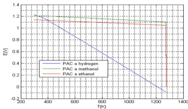
**Figure 3 :** Effect of temperature on EMF of FC (pure Oxygen P=1atm)
