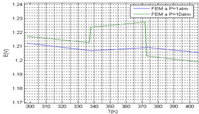
**Figure 5:** Effect of the temperature on the EMF of methanol FC for different pressure values (P=1atm et P=10atm pure oxygen)
