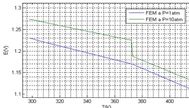
**Figure 6 :** Effect of the temperature of the EMF of hydrogen FC for different pressure values (P=1atm et P=10atm)
