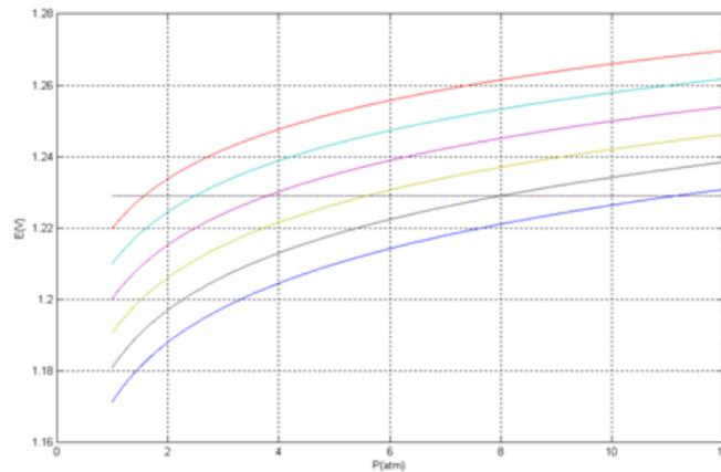
**Figure 8 :** The compensation pressure at different temperature values for FC with hydrogen (E = 1.23V)
