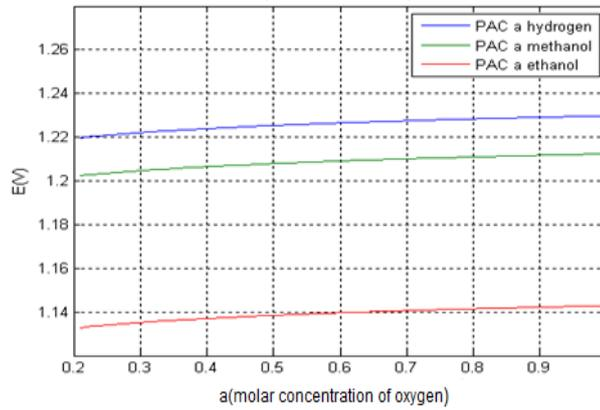
**Figure 1 :** Influence of the molar concentration of oxygen on the EMF (T = 298K P = 1atm)
