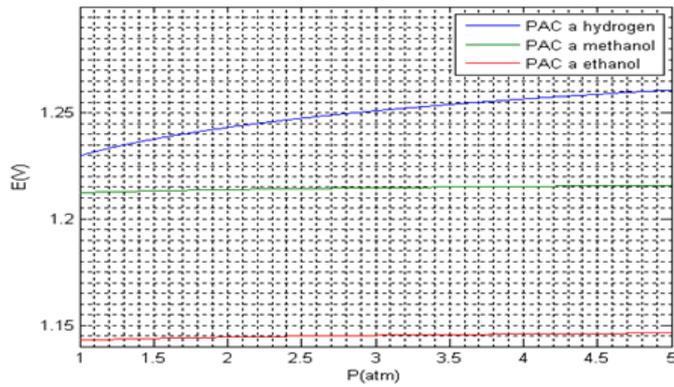
**Figure 7 :** Effect of the pressure on the EMF of FC (T=298K pure oxygen pure)
