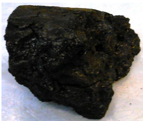
Figure 1: Sample of coking
