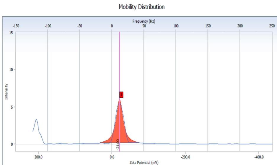
**Figure 5:** Zeta potential analysis of synthesized copper oxide nanoparticles.
