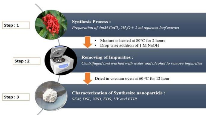
**Figure 1:** Graphical representation for formation of copper oxide nanoparticles.
