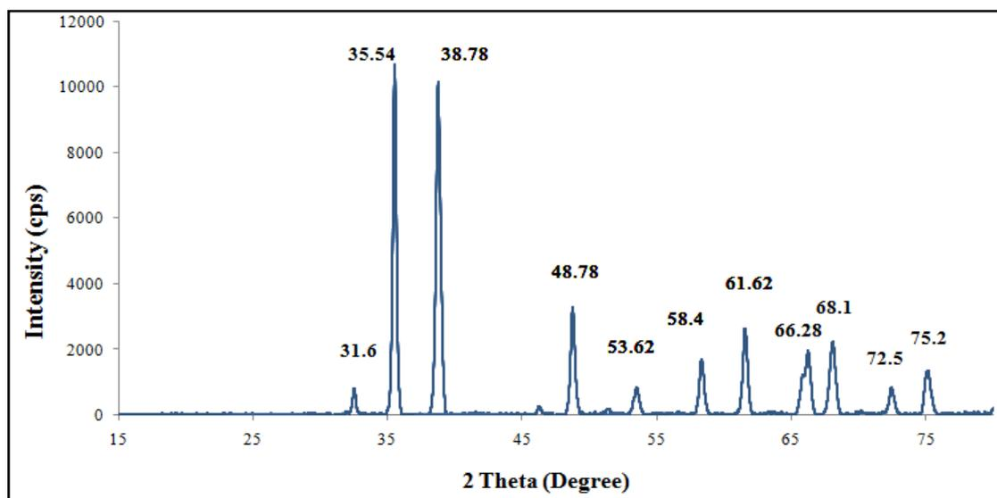
**Figure 3:** XRD pattern of synthesized copper oxide nanoparticles
