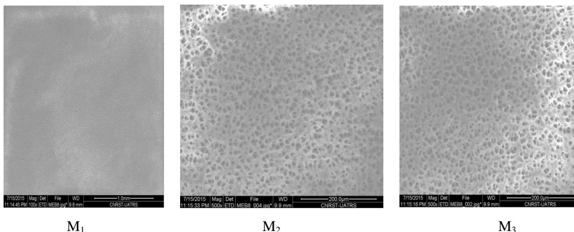
**Figure 5:** SEM photographs at various percentages % of  $\text{TiO}_2$
