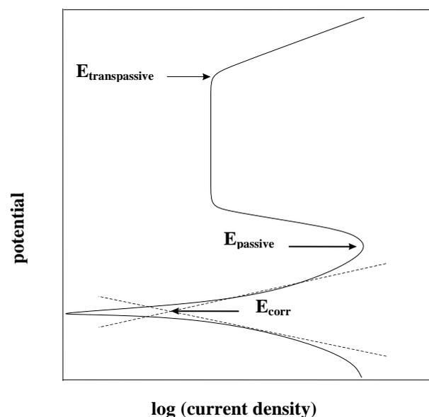
Figure 1: The determination point of  $E_{corr}$ ,  $E_{passive}$ , dan  $E_{transpassive}$
