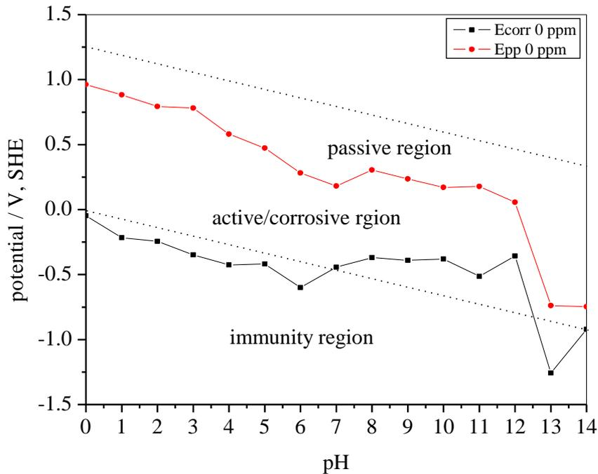
**Figure 3:** E-pH diagram in solution without BWP extract inhibitor in  $H_2SO_4$  system
