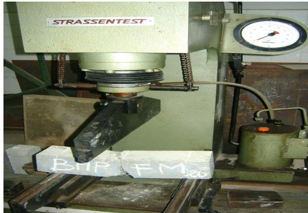
**Figure 8:** Machine of flexural strength.
