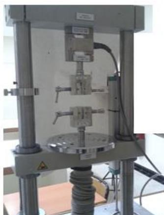
**Figure 5:** Tensile testing machine.
