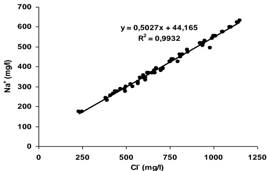
**Figure 3:** Correlation between the concentrations of Na<sup>+</sup> and Cl<sup>-</sup> ions.
