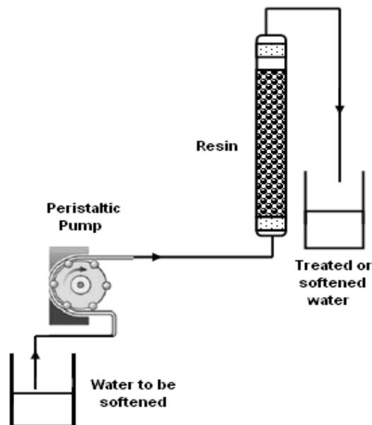
**Figure 1:** Scheme of the experimental system used in dynamic mode.
