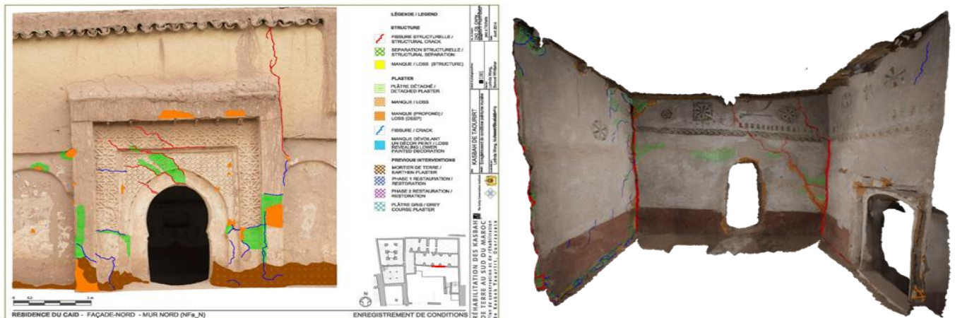
Figure 3 – Map of conditions in the Caid Residence (left), and 3D orthographic model of a painted room highlighting structural problems (right). Images: Lori Wong and Samuel Whittaker, 2014.
