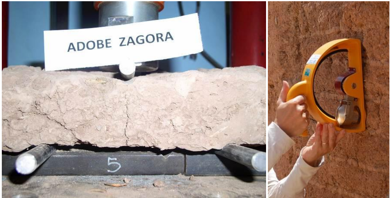
Figure 11: Sample F three point bending tests (left). Figure 12: Sclerometer tests on rammed earth wall (right).
