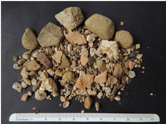
**Figure 4:** Pebbles and fragments of mortar, terracotta and wood in the rammed earth masonry of the wall D (PI500)
