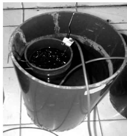
**Figure 3:** Design of the Sedimentation Microbial Fuel Cell (left) and real reactor (right) used in this study
