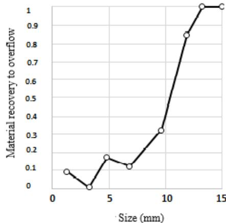
Figure 4- Partition curve of second deck of screen
