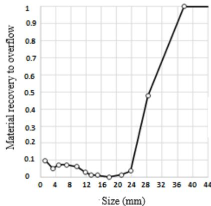
Figure 3- Partition curve of first deck of screen
