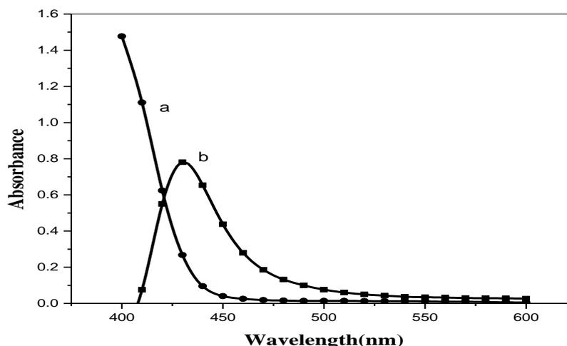
**Figure 4:** Absorption Spectra of a. PDT Vs Water blank, b. Ni(II) –PDT Vs PDT, Ni(II): 1.0 ml of  $4 \times 10^{-5}\text{M}$ , PDT: 1.0 ml of  $4 \times 10^{-4}\text{M}$ , pH:6.0,  $\lambda_{\text{max}}$  430 nm.
