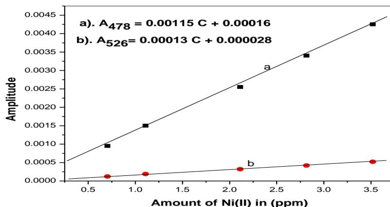
**Figure.11.** Second derivative amplitude Vs amount of Ni(II)  $\mu\text{g/ml}$ ; PDT:  $4 \times 10^{-4}$  M; pH: 6.0.
