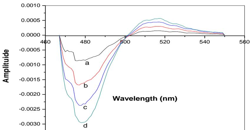
**Figure. 10.** Second order derivative spectrum of Ni(II)-PDT Complex; Nickel(II), ppm ; a. 0.704; b.1.408; c. 2.112; d. 2.816; PDT:  $4 \times 10^{-4}$  M; pH: 6.0.
