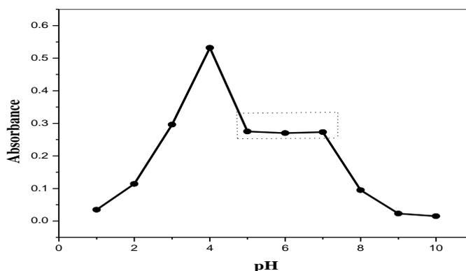
**Figure 5:** Effect of pH on the absorbance of Ni(II) –PDT complex, Ni(II): 1.0 ml of  $4 \times 10^{-5}$  M, PDT: 1.0 ml of  $4 \times 10^{-4}$  M,  $\lambda_{\max}$  430 nm.
