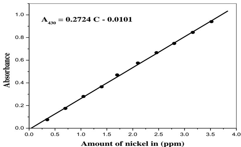
Figure.7. Zero order calibration plot for the Ni(II)-PDT system; Ni(II): 0.35-3.53 ppm; PDT:  $6 \times 10^{-6} M$ ; pH:6.0; max:430nm.
