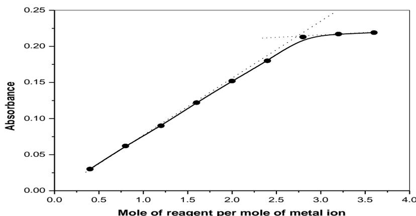
Figure. 9: Mole ratio method of Ni(II)-PDT Complex: Ni(II):  $2 \times 10^{-4}$  M; PDT:  $2 \times 10^{-4}$  M; pH:6.0;  $\lambda_{\max}$ :430nm.
