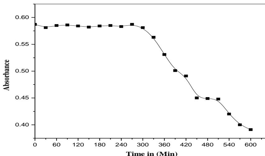
**Figure 6:** Time stability of the Ni(II)-PDT complex; Ni(II): $4 \times 10^{-5}$ M; PDT:  $4 \times 10^{-4}$ M; pH:6.0;  $\lambda_{\max}$ =430nm.
