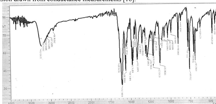
**Fig.1** IR spectrum of  $[\text{CuL}^2(\text{OAc})_2]$
