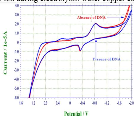
**Fig.4** Cyclic voltammogram of  $[\text{CuL}^6(\text{OAc})_2]$  complex in the presence and absence of different concentrations of DNA
