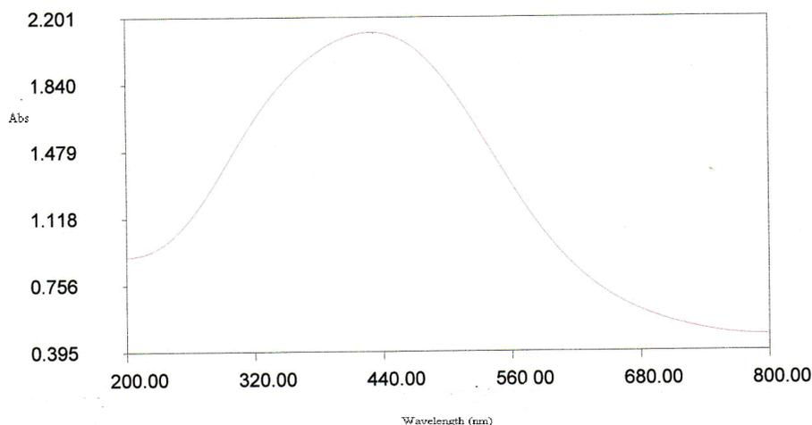
**Fig.2** Electronic spectra of  $[\text{CuL}^2(\text{OAc})_2]$
