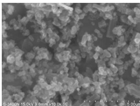
**Fig. 3** SEM image of  $[\text{CuL}^5(\text{OAc})_2]$  complex
