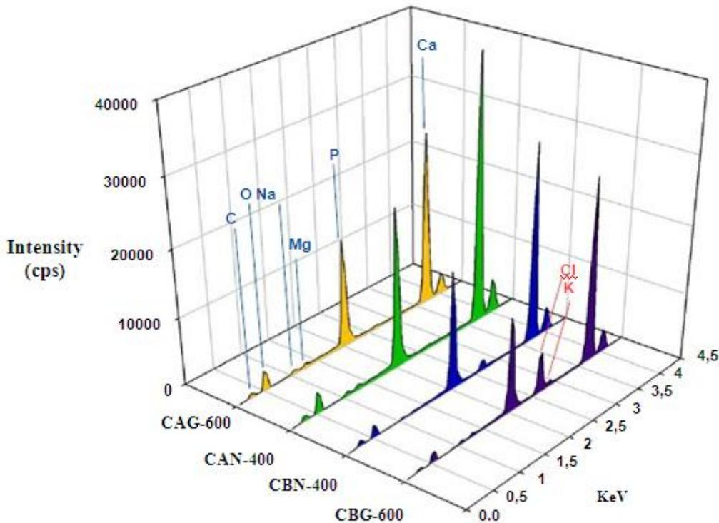
**Figure 2.** Representation of peaks of diffraction of the X-rays (EDX) in 3D of the various samples
