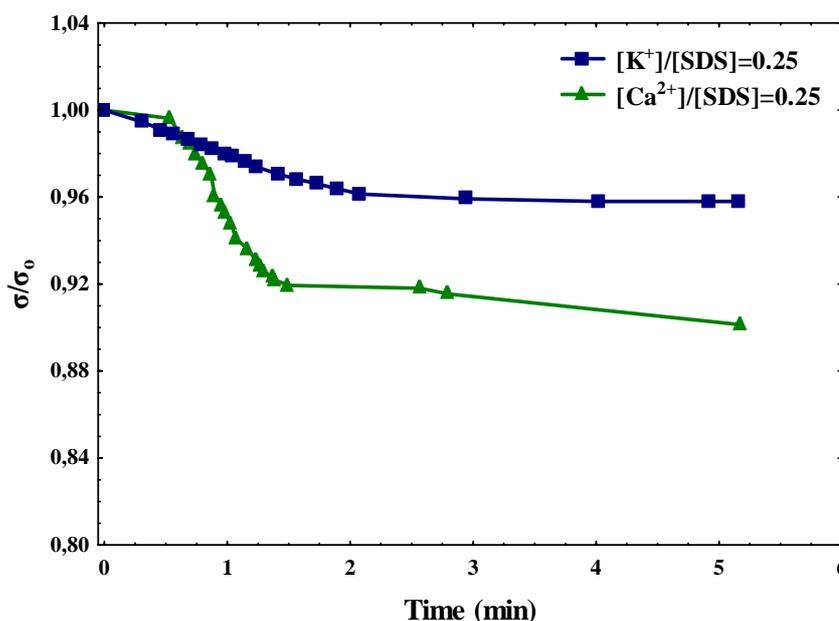
**Figure 4:** Normalized electrical conductivity time course during the precipitation of the SDS at 30°C using KCl and  $\text{CaCl}_2$  in presence of 1.2 mM of *p*-coumaric acid.
