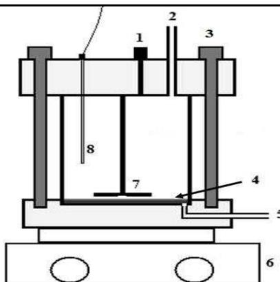
**Figure 1:** Scheme of the nanofiltration and ultrafiltration experimental set-up: 1. Feed inlet, 2. Connection to the nitrogen cylinder, 3. Screw, 4. Membrane, 5. Permeate outlet, 6. Magnetic stirrer, 7. Magnetic bar, 8. Temperature sensor.
