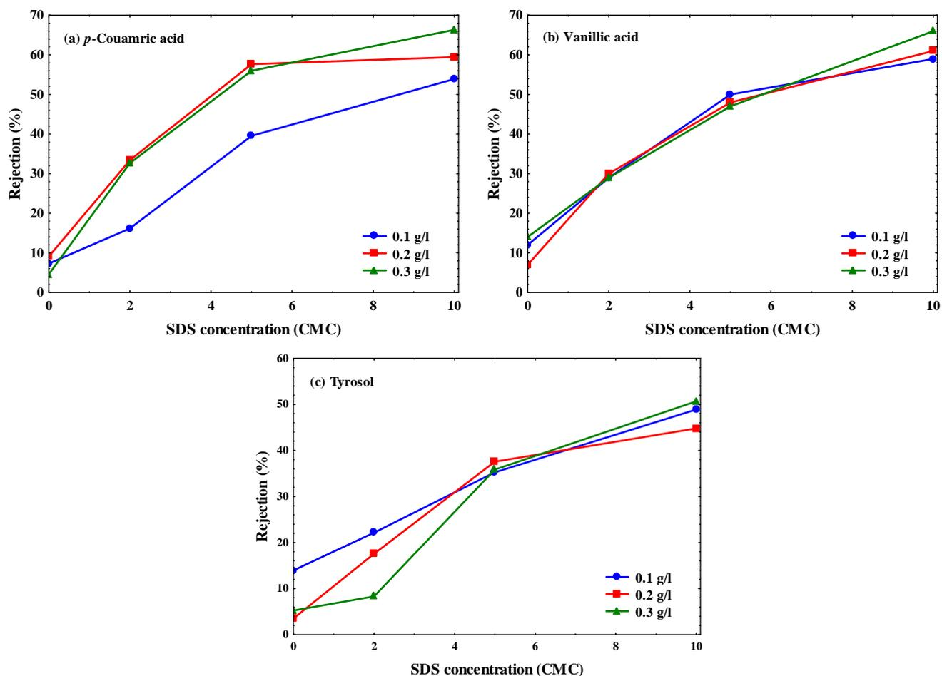
**Figure 3:** Rejection of phenolic compounds by MEUF against surfactant concentration for different model solutions using UF50 membrane: (a) *p*-coumaric acid, (b) vanillic acid and (c) tyrosol.
