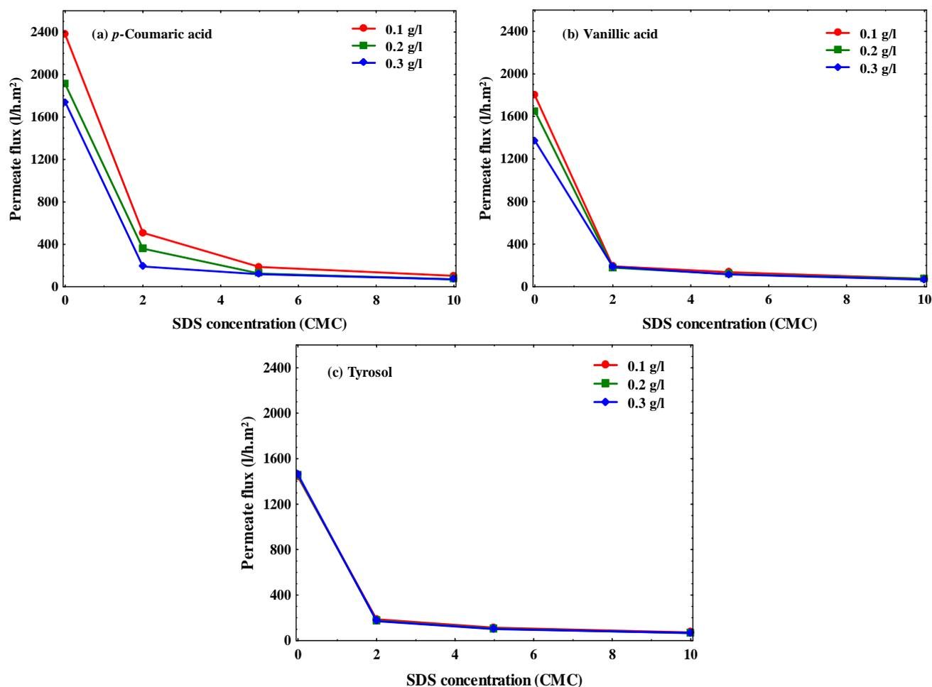
**Figure 2:** Permeate fluxes against surfactant concentration for the MEUF of different model solutions using UH050 membrane: (a) *p*-coumaric acid, (b) vanillic acid and (c) tyrosol.
