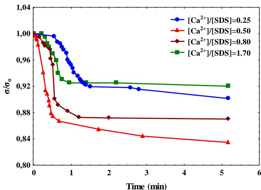
**Figure 5:** Normalized electrical conductivity time course during the precipitation of the SDS at 30°C using  $\text{CaCl}_2$  at different mole ratios in presence of 1.2 mM of *p*-coumaric acid.
