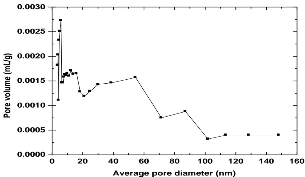
Figure 1: Pore size distribution of SBP obtained from BET analysis.
