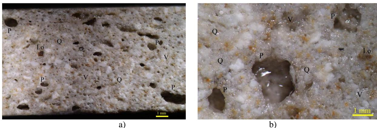
**Figure 4:** a) Optical micrographs showing the highly porous structure of the firebrick with 30% of expanded perlite. b) Detailed observation of pores systematically covered by glass products.
