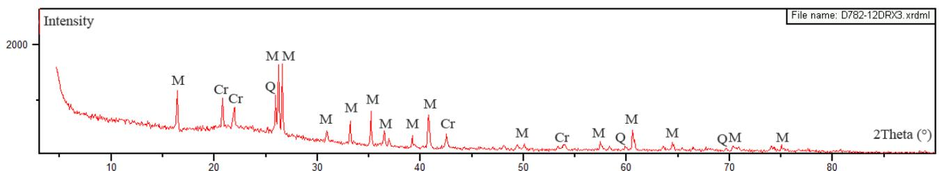
**Figure 2:** X-ray diffraction patterns of the brick manufactured from mixture and fired at 1600°C/1h (M: Mullite, Q: Quartz, Cr: Cristobalite) [13]
