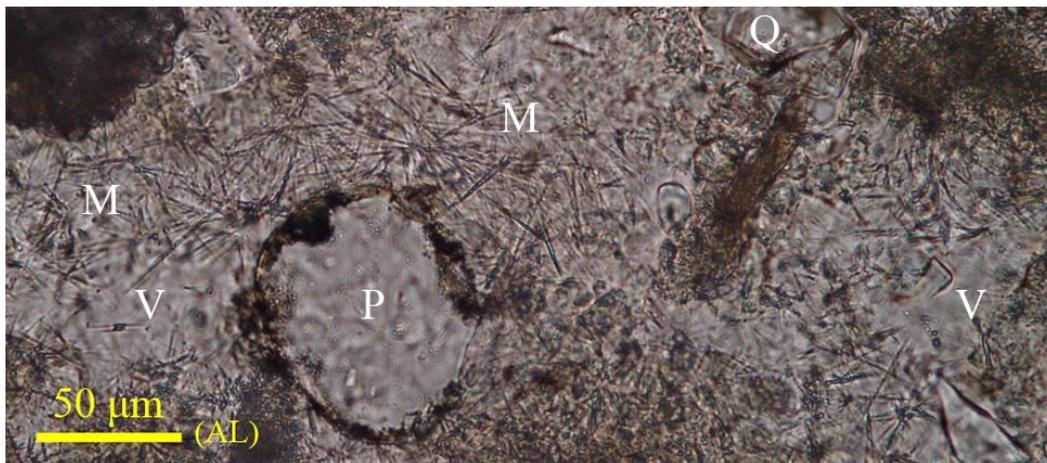
**Figure 6:** Micrograph showing the shape and abundance of mullite crystals invading the vitreous bottom of the firebrick (PL)
