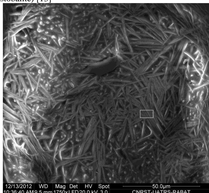
**Figure 3:** SEM microphotography of firebrick [13]
