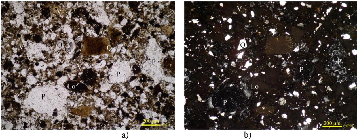
**Figure 5:** Microstructural analysis of the bricks taken with. a) Natural microscopy light (AL). b) Polarized microscopy light (APL). P: Porosity, I.o: Iron oxide, Q: Quartz, V: Vitreous phase.
