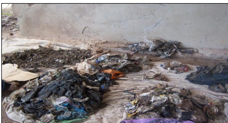
Fig. 5 Sorting of landfilled waste, into different components.
