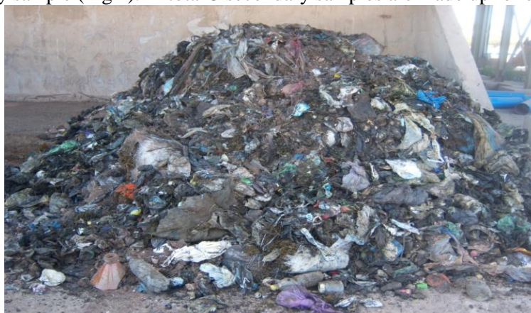
Fig. 4: Photo of landfilled waste piled in a hall reserved for the secondary sampling.
