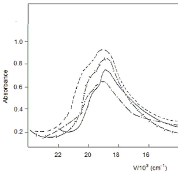
**Figure 3.** Electronic spectra of the original o-chloro (—) and o-bromo (-I-I-I) complexes and their thermal products (——) and (- - - - -), respectively.
