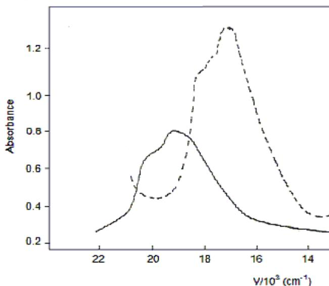
**Figure 5.** Electronic spectra of the original 2,4-dichloro complex (—) and its thermal blue thermal product (----).
