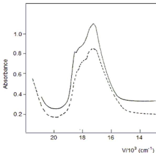
**Figure 4.** Electronic spectra of the original 2,4-dimethyl complex (—) and its thermal product (----).
