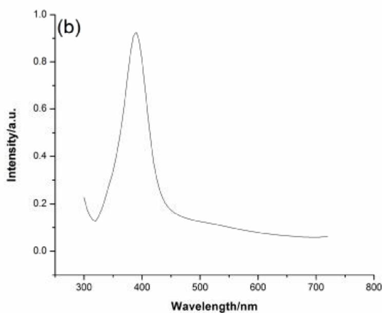
**Figure 1:** TEM (a) and UV-Vis spectrum (b) of synthesized nanosilver using Tollens' method (Black line=200 nm).
