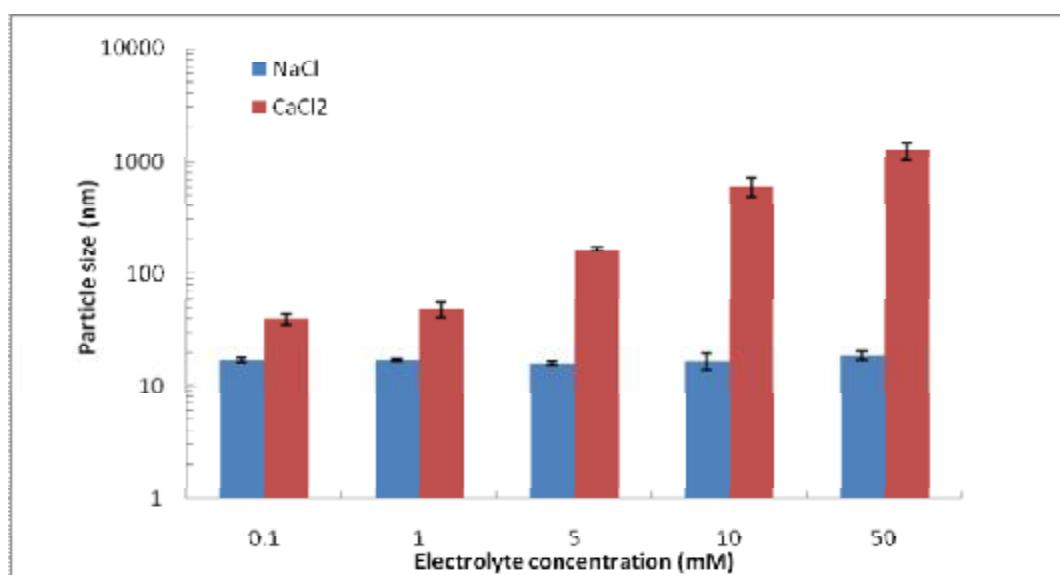
**Figure 4:** Particle size of nanosilver in different electrolyte solutions.
