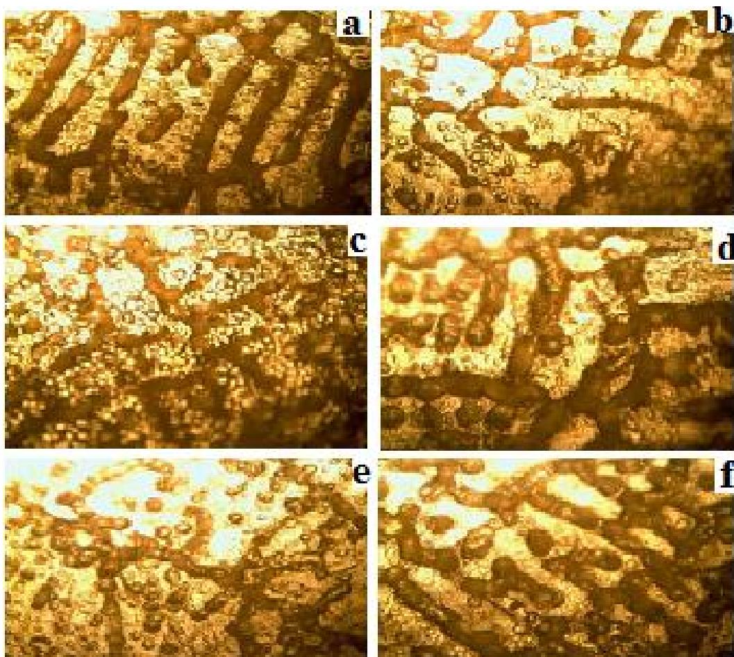
**Figure 4:** Microstructure of cast Al-Si-Mg alloy (a) solution heat treated at 540°C/1 h (b) aged for 1 h (c) 2 h (d) 3 h (e) 4 h (f) 5 h       $\times 100$
