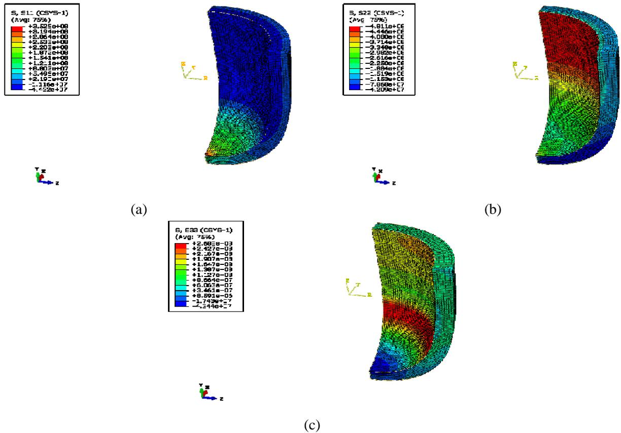
**Figure 6:** Stress contours with aluminum liner: a) radial direction; b) tangential direction; c) along the main axis element
