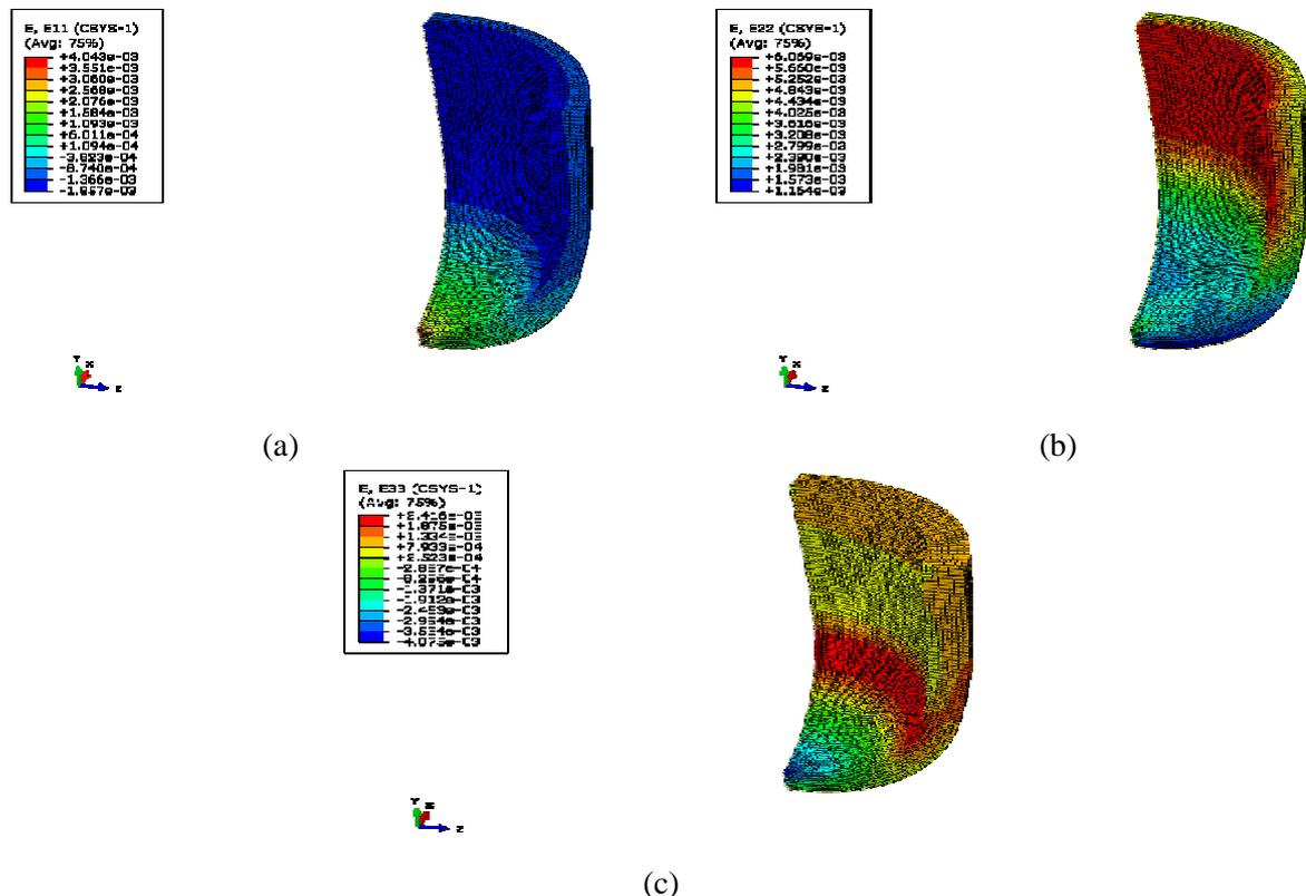
**Figure 7:** Strain contours without aluminum liner: a) radial direction; b) tangential direction; c) along the main axis element
