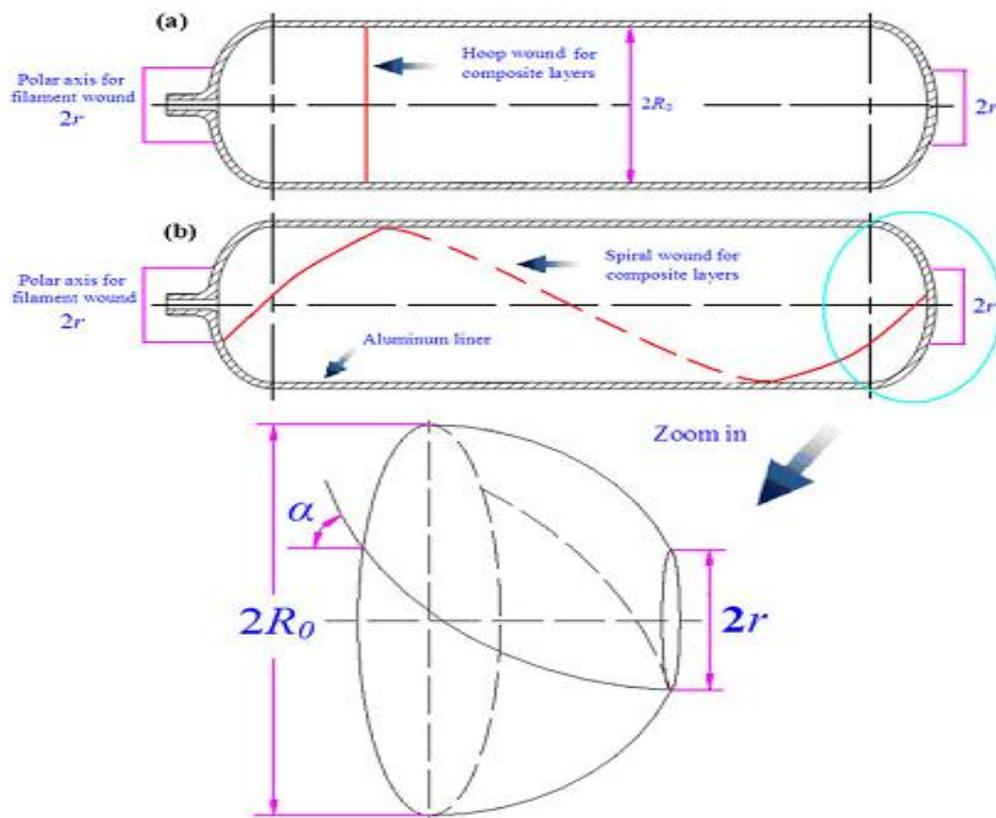
**Figure 3:** Basic structure and wound pattern of composite vessel: (a) hoop wound; (b) spiral wound [7]
