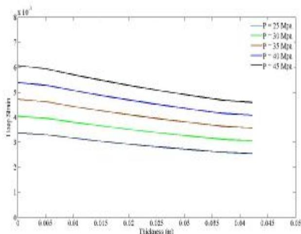
**Figure 10:** Effect of vessel thickness and pressure on hoop strain
