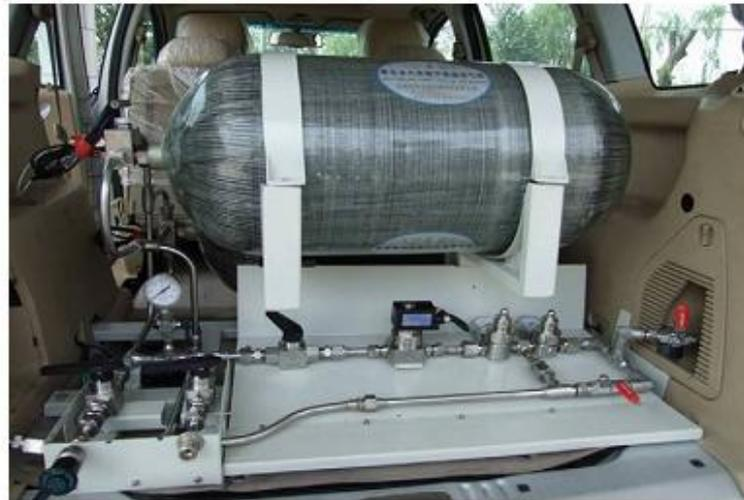
**Figure 2:** Lightweight composite high-pressure hydrogen storage vessel used in the hydrogen fuel-cell vehicle [7].
