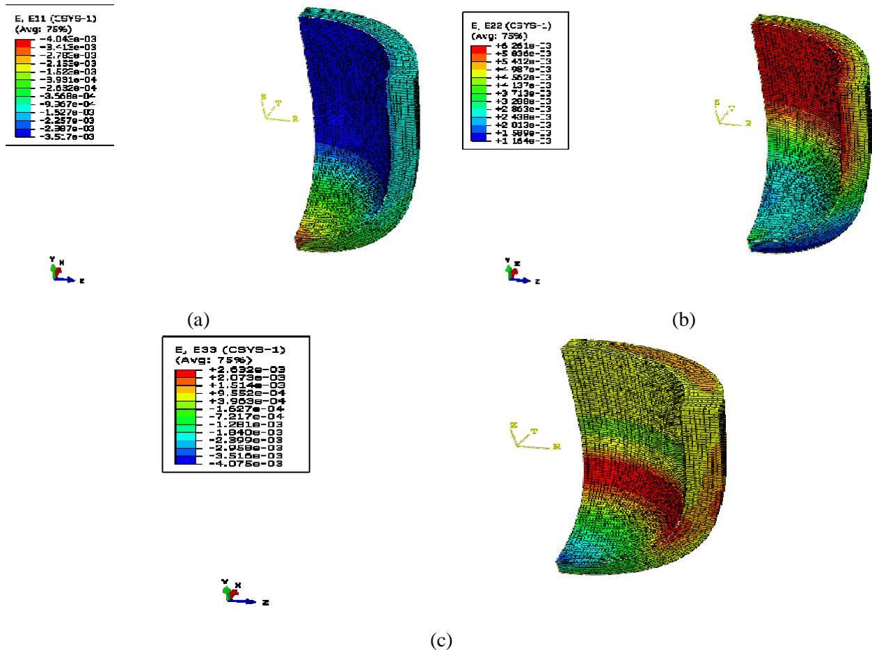
**Figure 8:** Strain contours with aluminum liner: a) radial direction; b) tangential direction; c) along the main axis element
