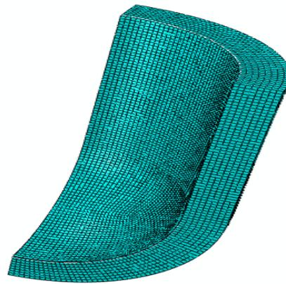
Figure 4: Finite element model of composite vessel
