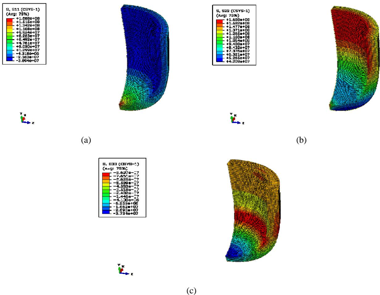
Figure 5: Stress contours without aluminum liner: a) radial direction; b) tangential direction; c) along the main axis element
