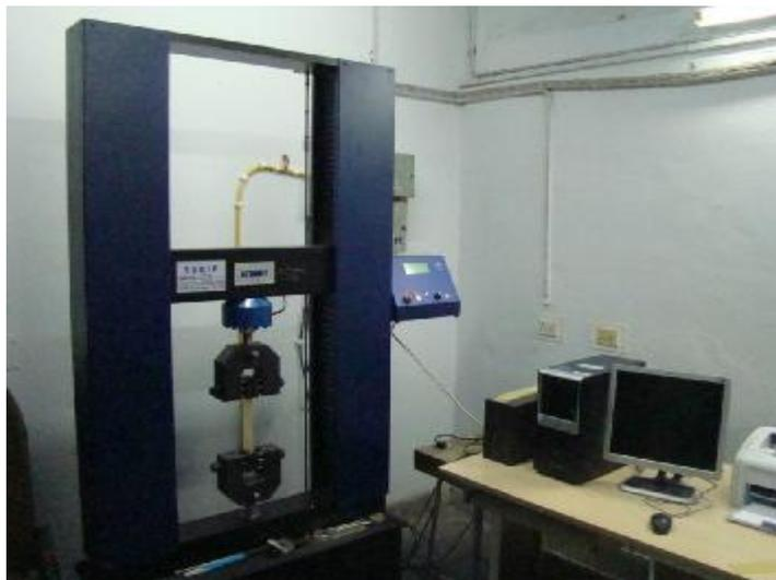
**Fig. 3:** Universal Testing Machine
