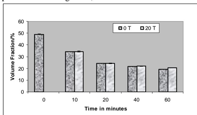
**Figure 1:** Changes in Beta Fiber Volume Fraction for Samples Heat Treated at 350°C.
