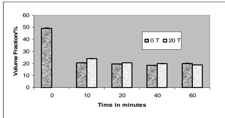
**Figure 2:** Changes in Beta Fiber Volume Fraction for Samples Heat Treated at 400°C.
