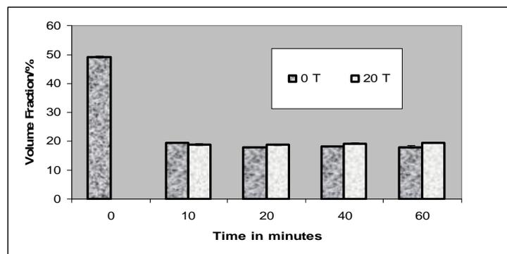
**Figure 3:** Changes in Beta Fiber Volume Fraction for Samples Heat Treated at 450°C.
