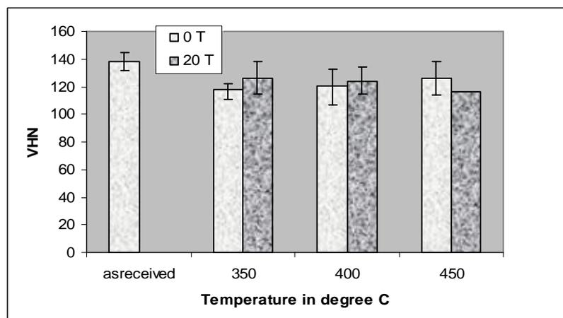
**Figure 4:** Temperature Effect on Microhardness values for 40 minutes.
