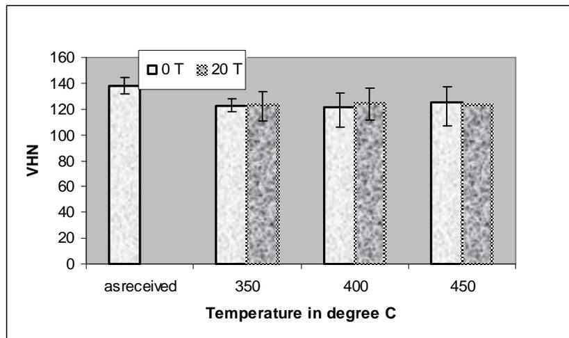
**Figure 5:** Temperature Effect on Microhardness values for 60 minutes.
