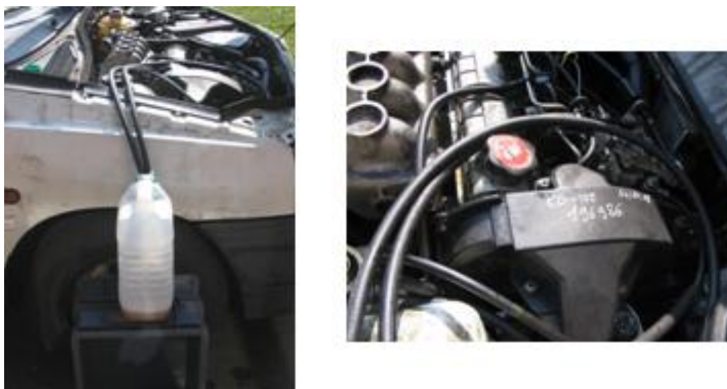
Figure 1: view of the external tank and of the fuelling lines
