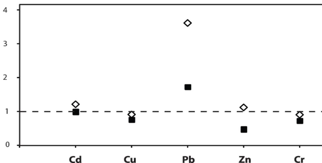
**Figure 5:** Comparison of the Tomlinson Pollution Load Index (PLI) of analyzed heavy metal concentration (Cd, Cu, Pb, Zn and Cr) in the topsoils in parcel 1 (light diamond) and parcel 2 (dark square).
