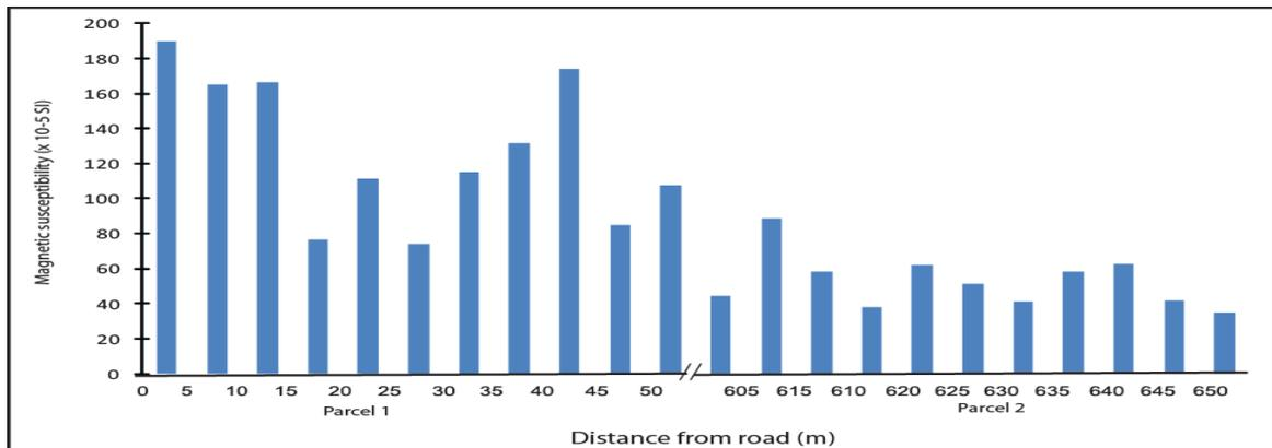
**Figure 2:** Histogram plot showing magnetic susceptibility variation versus distance from road and automotive exhausts
