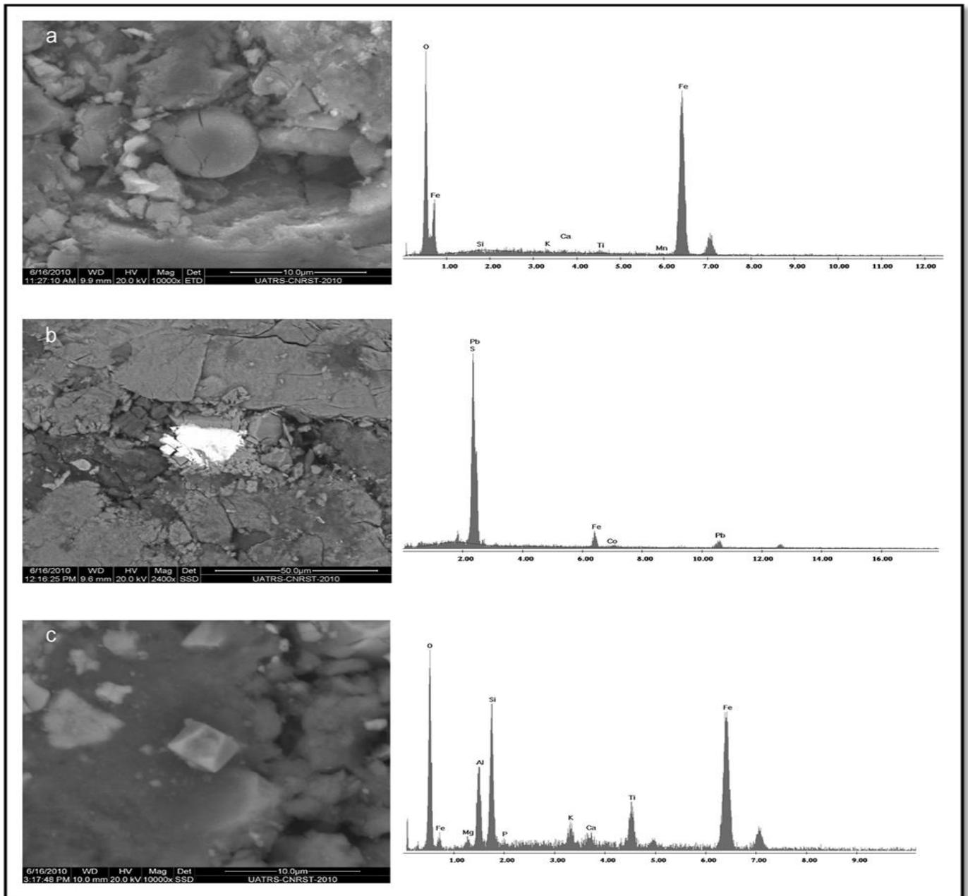
**Figure 6 :** Scanning electron micrograph (SEM) with corresponding energy spectra of extracted magnetic fractions in parcel (1) with spherule form (a) and in parcel (2) showing Pb spots (b) and titanomagnetite octahedron associated with silicates (c).
