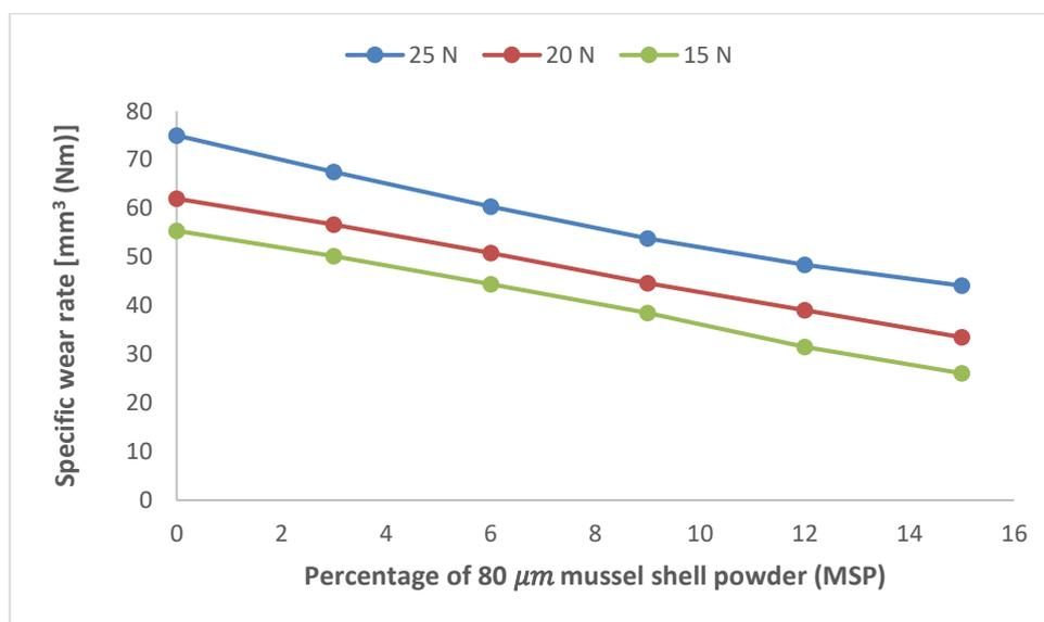
Figure 8. Effect of reinforcement on specific wear rate
