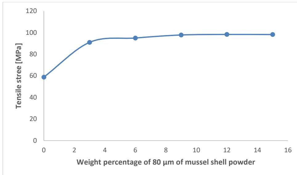
**Figure 4.** Variations of tensile stress of Alloy and composites against wt. % MSP
