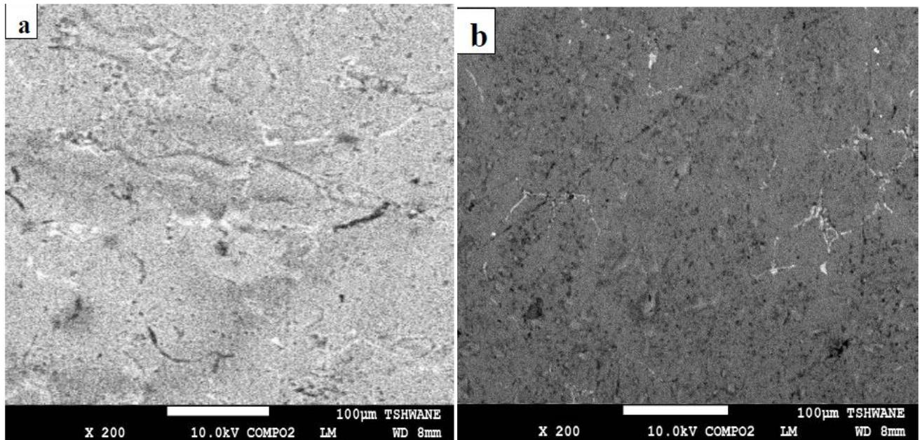
**Figure 3.** The morphologies of (a): Al-0.7% Mg-0.4 % Si, (b): Al-0.7% Mg-0.4 % Si/12 wt. % MSP
