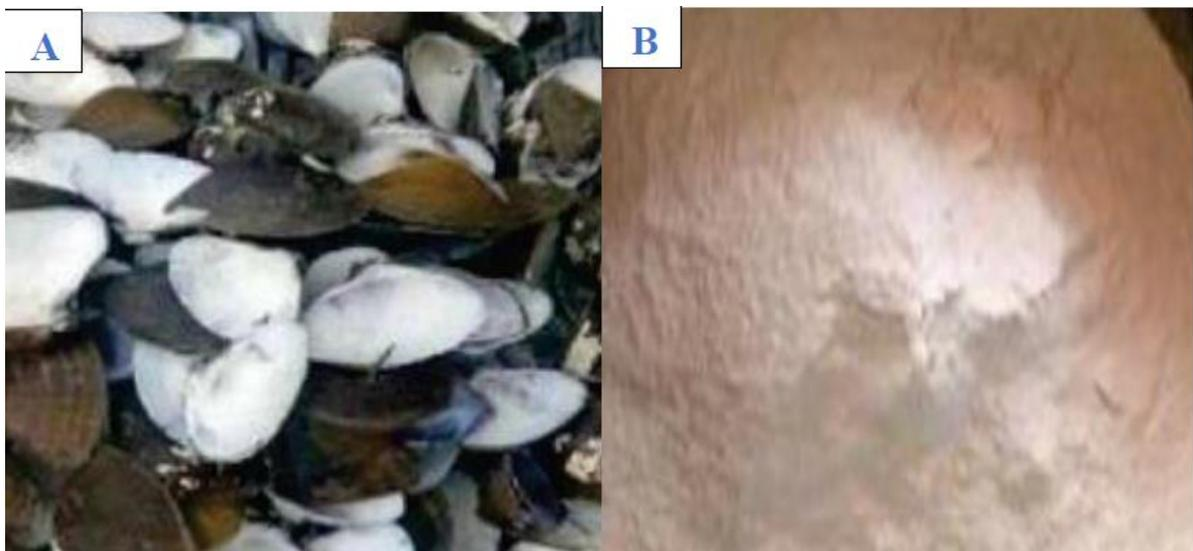
**Figures 1a and 1b.** (A) Mussel shell collections, and (B) mussel shell of particle size of 80  $\mu\text{m}$
