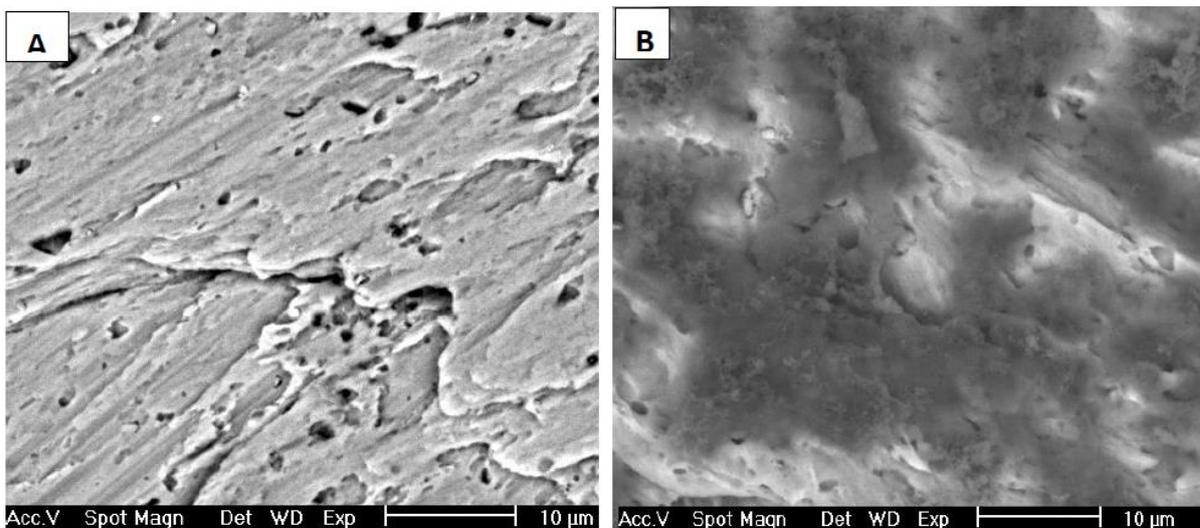
Figure 9. (a)-Morphology of Aluminium alloy 6063 without loads (b) – Alloy 6063 reinforced with optimum 15 wt. % of 80 µm MSP particles at different loads
