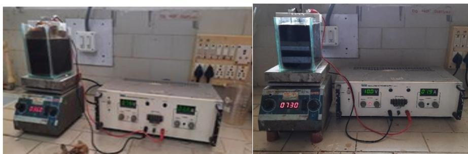
**Fig:1.** (a) Experimental setup of EC in lab scale with 2 electrodes of Stainless steel
