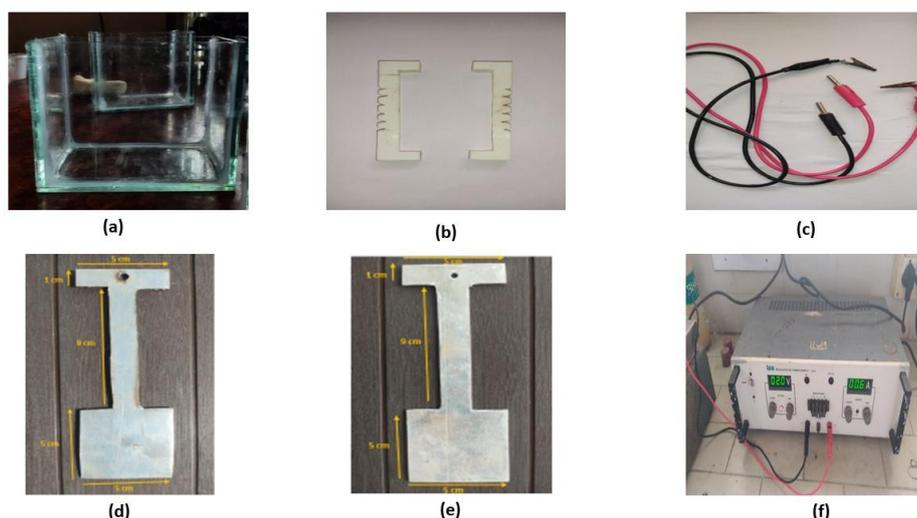
**Fig 2.** (a) Glass reactor, (b) Electrode holder, (c) Wire for DC connection, (d) Stainless steel Electrode (e) Aluminium Electrode, (f) DC Power supply
