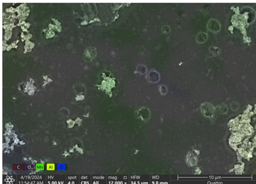
Figure 6: EDS obtained after analysis of the SEM deposit of the sample.
